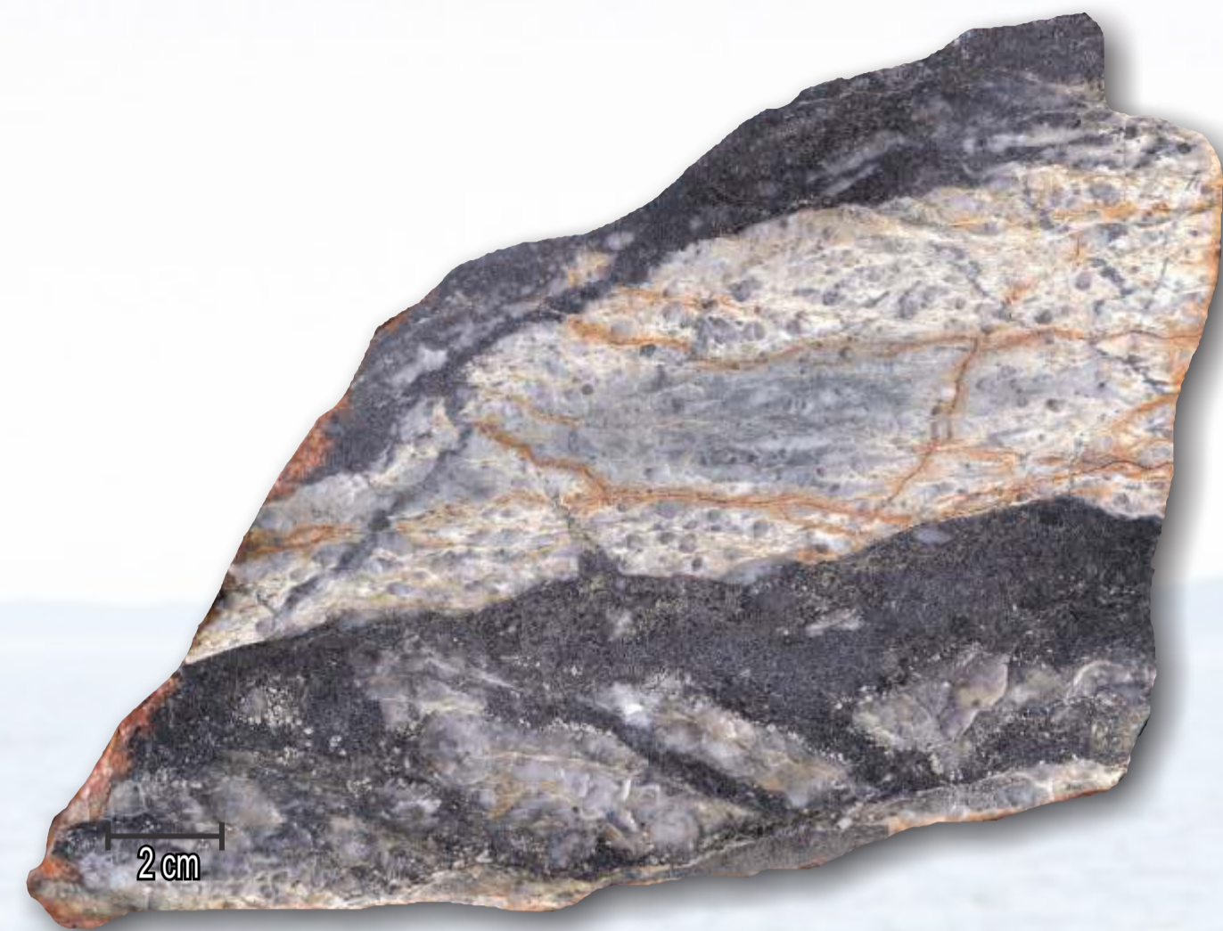
Quartz-phyric felsic volcanic host to the Katie VMS occurrence. This sample (15JH070) contains 11.1% Zn, 5.4% Pb, 0.3% Cu, 149 ppb Au and 31.8g/t Ag. Alteration is composed of silica-sericite-pyrite. Alteration indices: Alteration Index of Ishikawa et al. (1976) AI = 90, chlorite-carbonate-pyrite index of Large et al., (2001) CCPI = 81.
