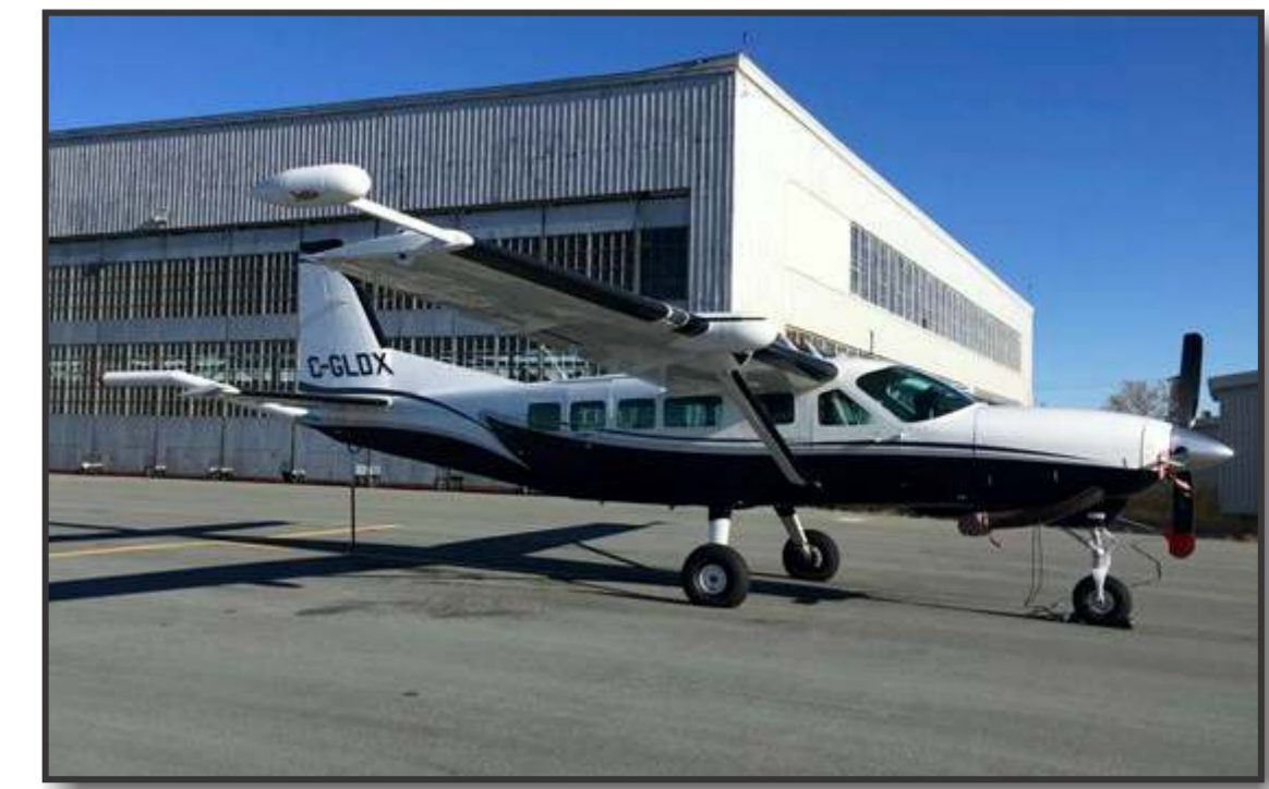
Figure 2: Goldak's Cessna Caravan aircraft equipped for airborne survey
