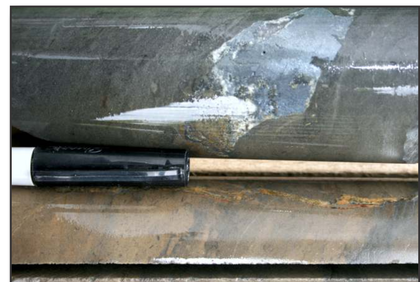
Stibnite and ankerite filling a late, fracture-related vug in interbedded grey sandstone and siltstone of the Indian Islands Group in diamond-drill hole BB11-228 (337.81m).
