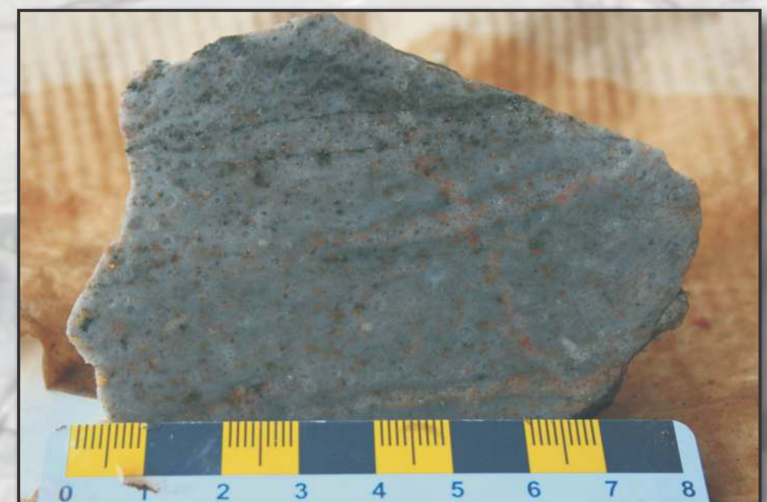
Intensely altered felsic metavolcanic rock of the Aillik Group, ca. 2 km from the Michelin deposit.
