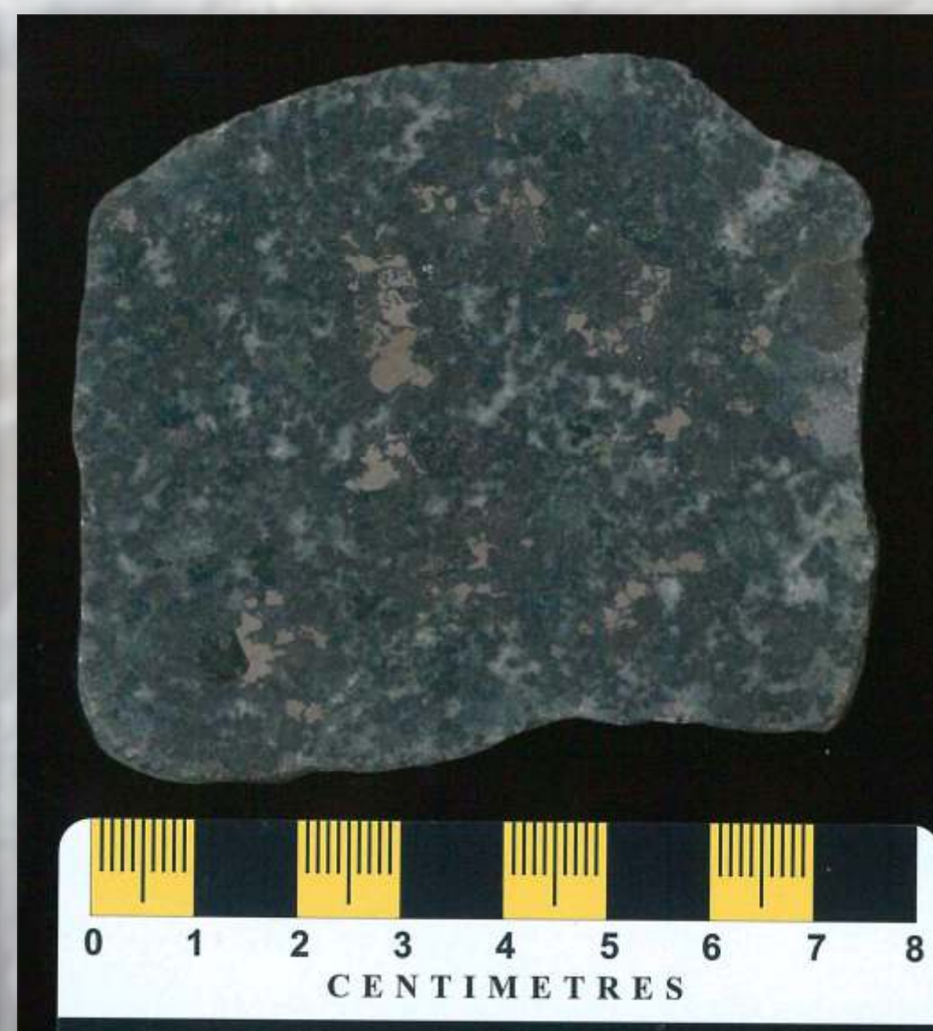
Medium grained gabbro from the Howse Lake area, with disseminated interstitial sulphides (pyrrhotite and minor chalcopyrite)
