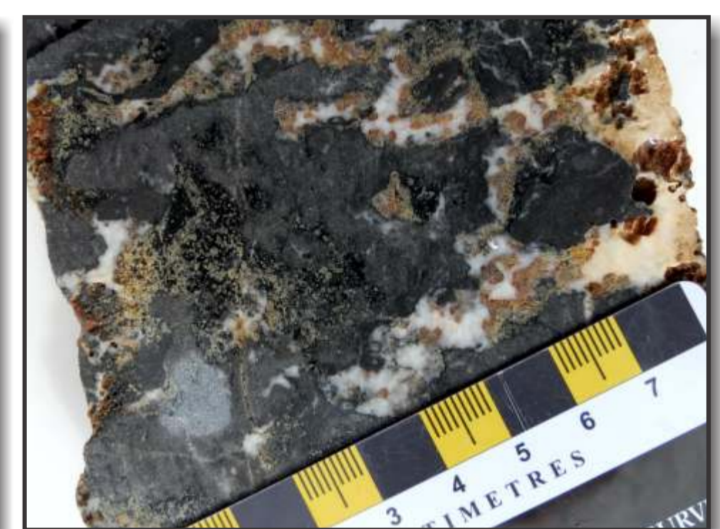
Mineralized boulder from Salmon River 6 Prospect, with red sphalerite associated with calcite and later yellow sphalerite associated with black quartz
