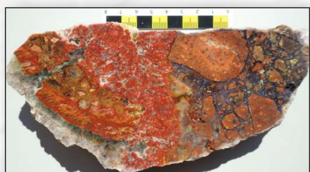
Hydrothermal breccia composed of sill clasts in purple fluorite matrix, surrounded by chert (fibrous chalcedony with Fe-oxide) with white fluorite, followed by the formation of green and white fluorite from the Open Cut Pit
