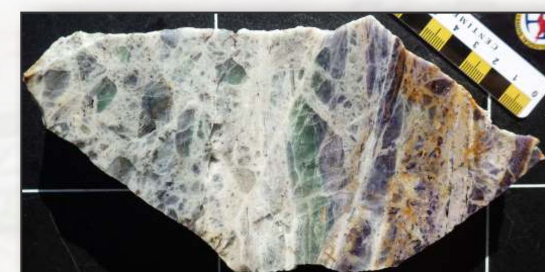
"Blastonite" composed of purple, green, blue and white fluorite in quartz rich matrix, representing the last phase of ore formation (Grebes Nest Pit)
