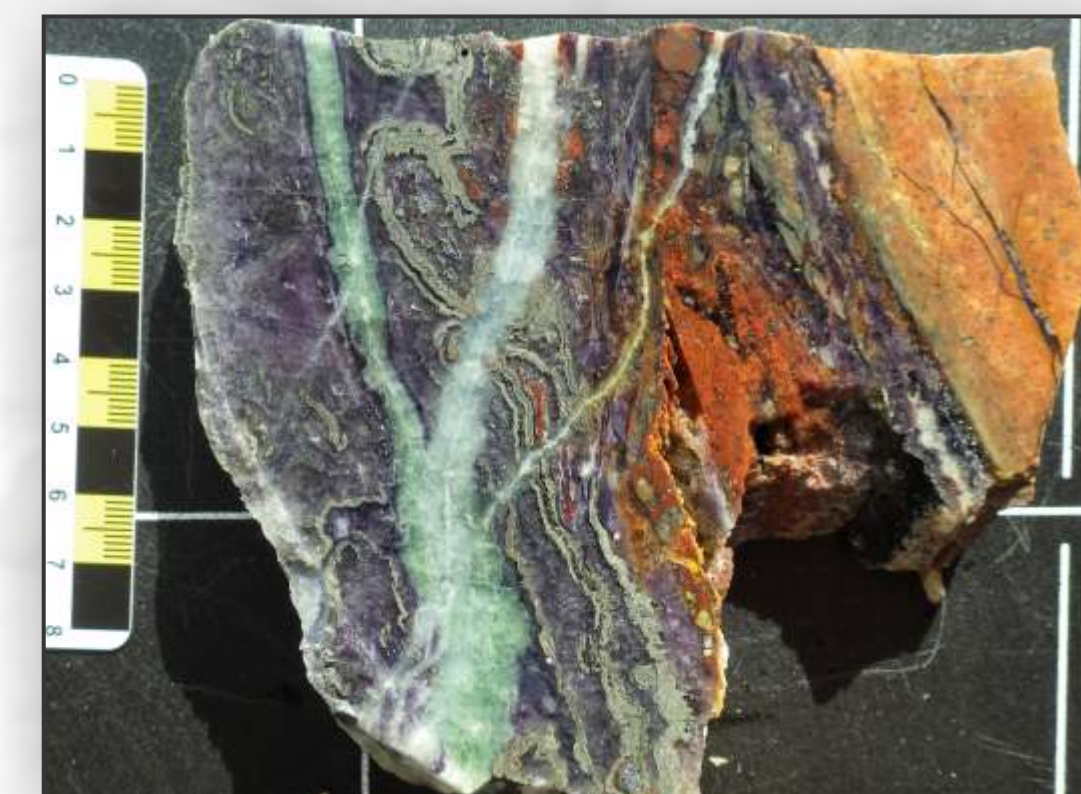
Purple fluorite in rhyolite sill followed by colloform banding of purple fluorite, galena and sphalerite, cut by green fluorite vein, which is cut by blue fluorite vein (Grebes Nest Pit)
