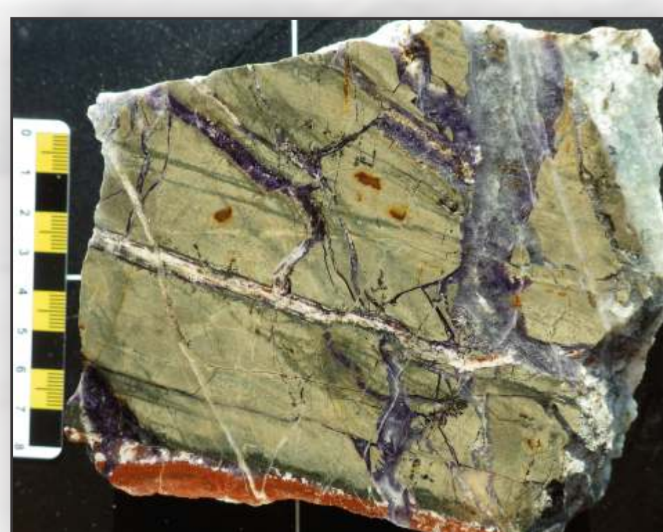
Stockwork purple fluorite at the contact of rhyolite sill and sediments, cut by blue fluorite and white calcite veins (Grebes Nest Pit)
