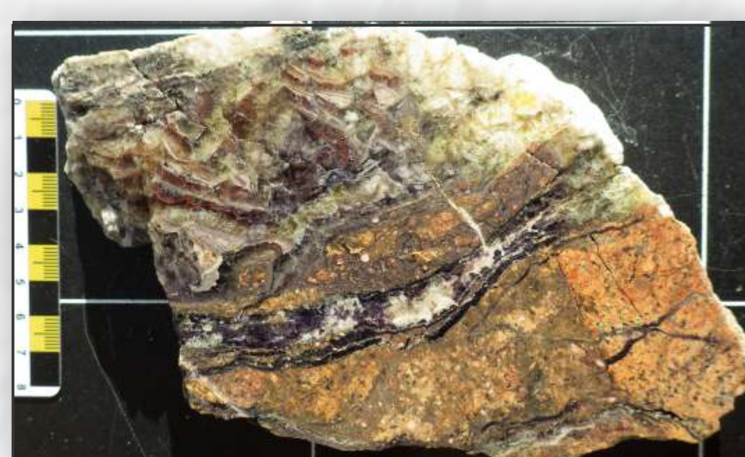
Purple fluorite with calcite (white), followed by the formation of colloform bands of yellow-green and red fluorite (hematite) in granite from Little Salt Cove vein
