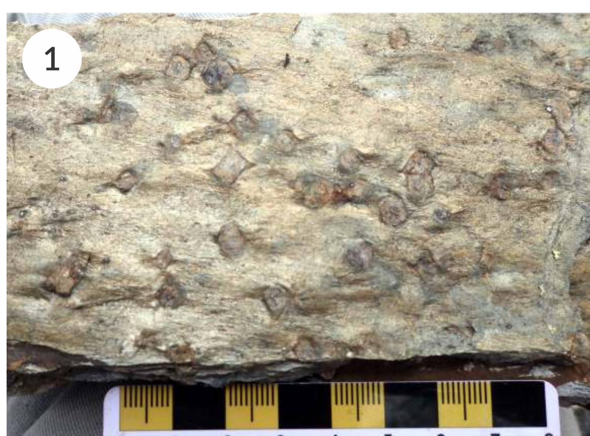
1 Garnet porphyroblasts, indicative of greenschist-facies metamorphic conditions, in lower KS phyllite. Metamorphic grade decreases to the west.
