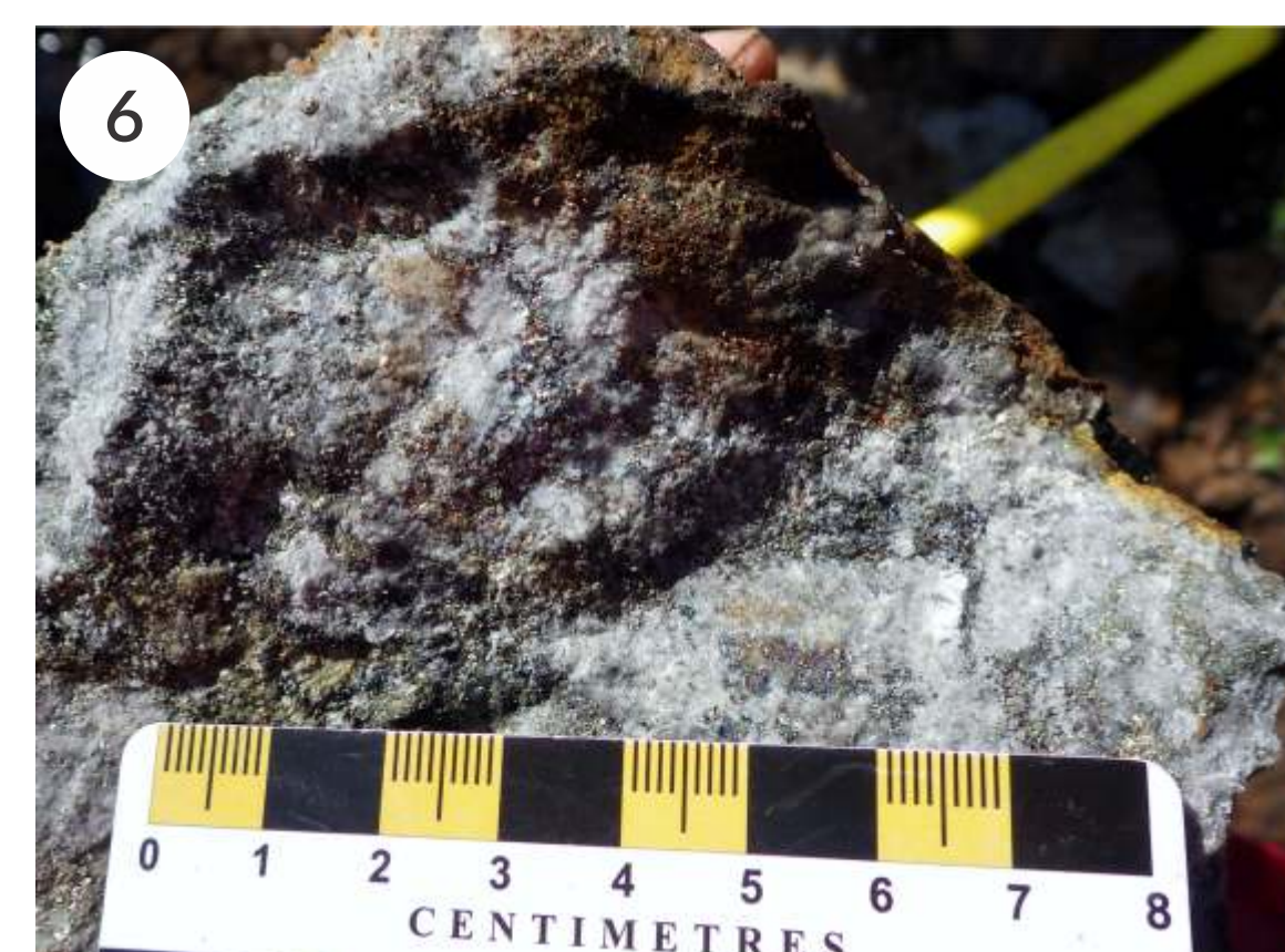
6 Silica-altered meta-sedimentary rock from the Menihek Formation (Ferriman Group) showing chalcocopyrite and bornite mineralization.
