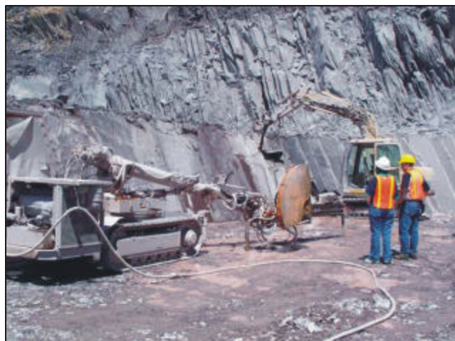
Plate 33. Rotary saws used to extract slate from the Britannia Cove quarry.
