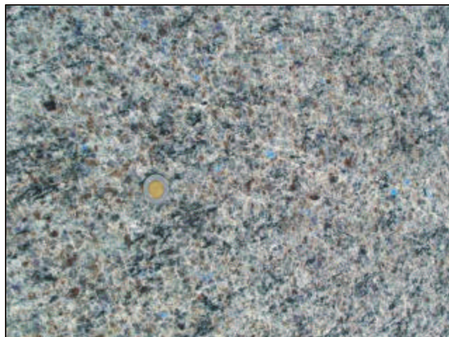
Plate 18. Polished slab of Ten Mile Bay anorthosite showing the blue iridescence or chatoyancy which gives the stone its trade name "Blue Eyes". Coin is 2.7 cm. in diameter.
