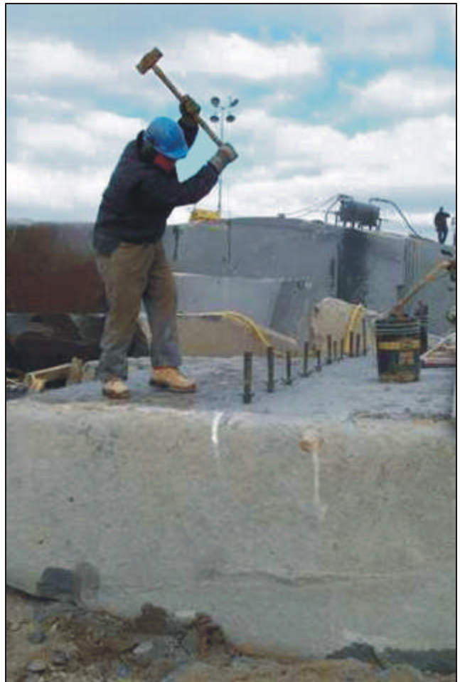
Plate 31. Splitting a large block into production blocks using plug and feathers, Finger Pond quarry, Jumpers Brook.
