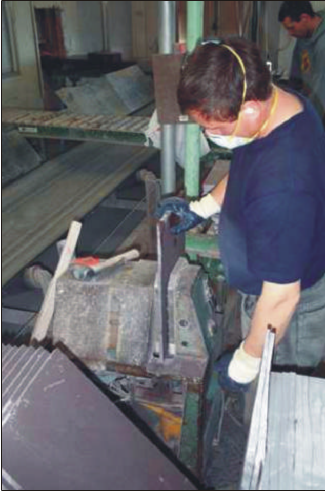
Plate 34. Splitting slate with hydraulic splitters, Hurley Slateworks Company, Britannia Cove, eastern Newfoundland.
