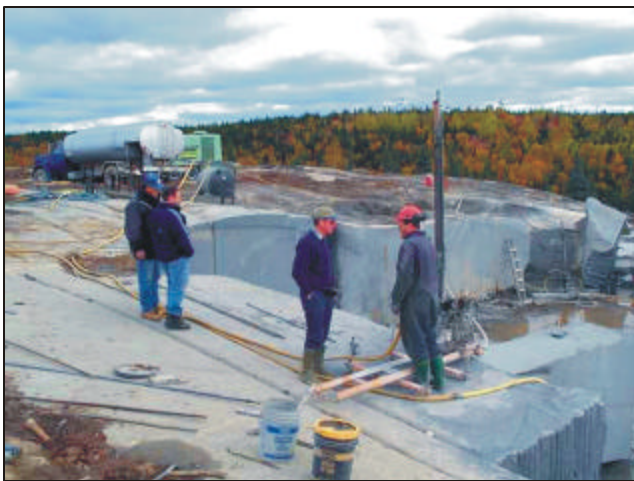
Plate 29. Quarry bar setup, Finger Pond quarry, Jumpers Brook, central Newfoundland.
