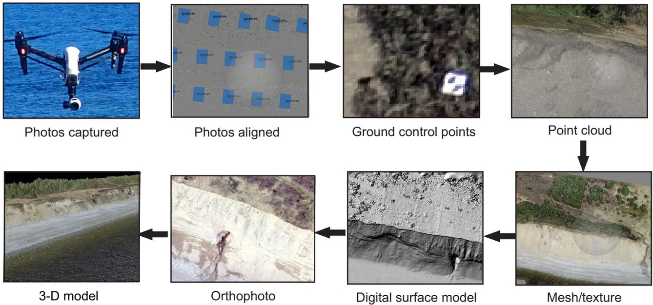
**Figure 3.** Workflow for collecting and processing aerial data. Aerial images are collected by UAV, and downloaded into a photogrammetry program. Next, the photos are aligned, and ground-control data imported. A point cloud, mesh and texture of the field site are created. Finally, a DSM, orthophoto and 3-D model are constructed.
