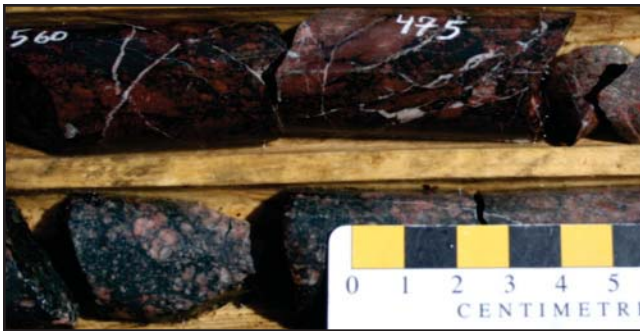
Plate 8. Cataclasite hosting uranium-bearing hematized quartz monzodiorite-tonalite fragments within a chlorite-rich breccia matrix; note that the breccia is crosscut by later carbonate veins (Anomaly No. 7 prospect; DDH 51544, ~45 m depth).
