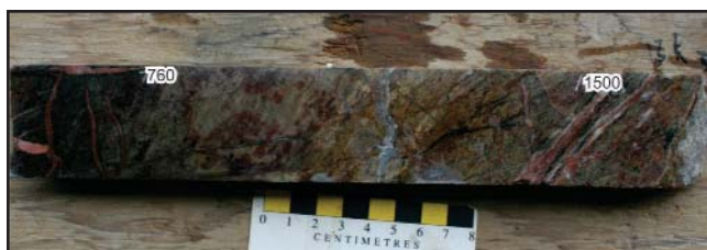
Plate 96. Uraniferous hematite-carbonate veins crosscutting reduced sandstone, Moran Heights prospect (DDH ML-MH-13, 36.5 m depth); white labels denote counts per second.
