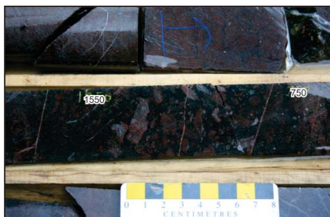
Plate 101. Uranium-bearing breccia located along the intrusive margin of a leucogabbroic dyke; B Zone prospect. A sample from this interval returned 0.34% U 3 O 8 , 0.12% V 2 O 5 , 0.25% Cu and 14.3 g/t Ag over 0.5 m (Sample #90838; Morgan et al., 2007; DDH ML-BZ-04, ~43 m depth); white labels denote counts per second.
