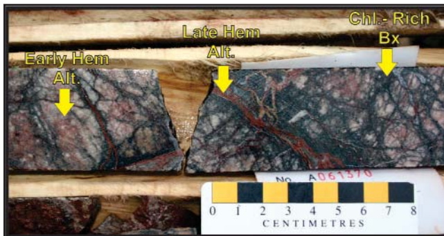
Plate 22. Early pinkish-red hematite (Early Hem) alteration crosscut by chlorite (Chl. Rich Bx)-rich brecciation overprinted by later hematite alteration (Late Hem); all phases are barren with respect to uranium mineralization; Two-Time deposit, DDH CMB-07-07, ~200 m depth.
