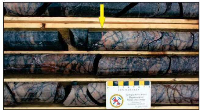
Plate 14. Fine-grained tonalite intruding weakly banded, chlorite-rich, gneiss. Note the well-developed fracturing and associated brecciation within the tonalite unit; Two-Time deposit, DDH CMB-07-14, ~160 m depth.
