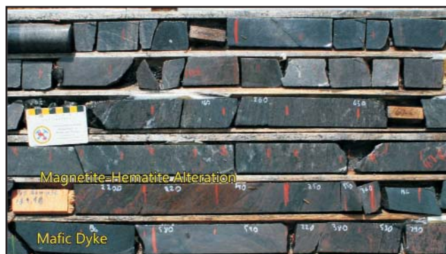
Plate 84. Photograph displaying a portion of the mineralized intersection in hole SP-06-10, which returned 0.12% U_3O_8 over 9.11 m; Mustang Lake area. The most significant zones of mineralization are associated with intense magnetite–hematite alteration. (White numerics denote cps as determined using a handheld scintillometer.) Mineralization is also locally crosscut by post-mineralization mafic dykes.
