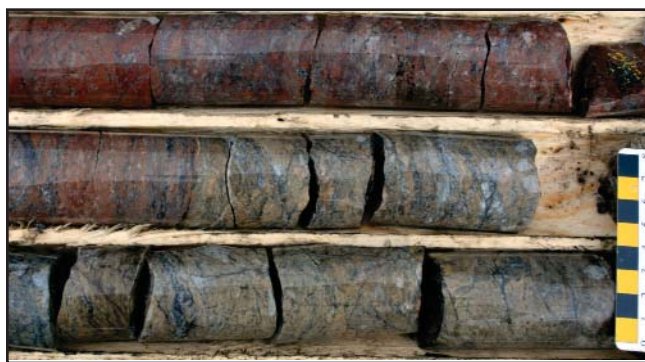
Plate 39. Pinkish-red hematite–carbonate–albite alteration flanked by pale-beige Fe-carbonate–albite alteration within altered argillite; note the highly disrupted nature of the host rock due to the structural control of the mineralization. Armstrong deposit, DDH MLAR-04, ~280 m depth.
