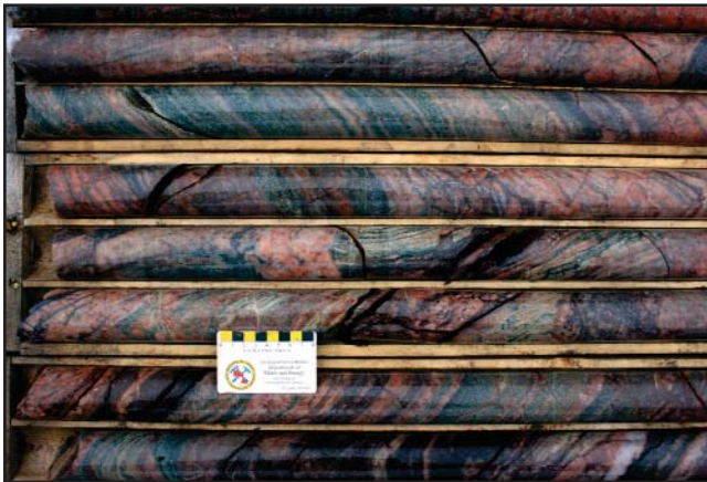
Plate 13. Well-developed banding in the Maggo Gneiss displaying local folding of the gneissic banding, crosscut by a late pegmatite dyke; Two-Time deposit, DDH CMB-07-21, ~440 m depth.
