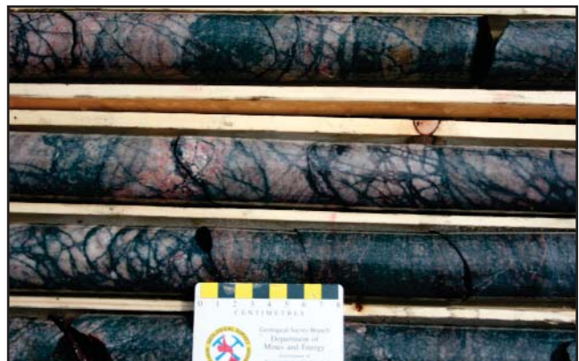
Plate 20. Development of the chlorite-rich ‘mega breccia’ within Maggo Gneiss marginal to the main mineralized zone; Two-Time deposit, DDH CMB-07-14, ~205 m depth.
