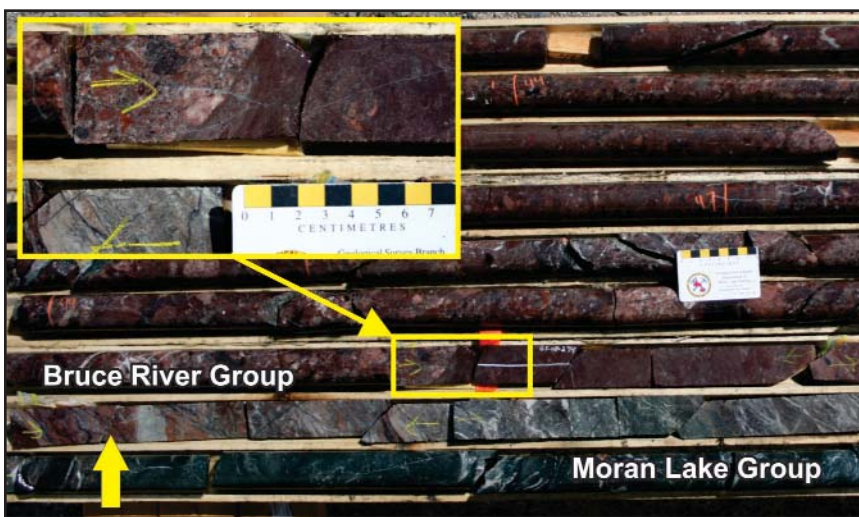
Plate 26. Hematite–albite–carbonate alteration (stubby yellow arrow) developed within metres of the overlying conglomerate of the Heggart Lake Formation. Note the sharp structural contact separating the two units (see inset). Moran Lake C Zone, DDH ML-56, ~50 m depth.
