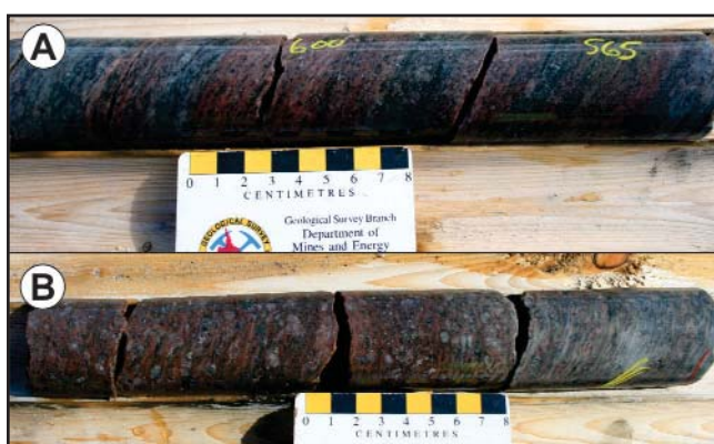
Plate 70. Typical features of mineralized core from the Michelin deposit illustrating the light-coloured (albitized) and red (hematized) metavolcanic host rock. A. Sub-porphyritic metavolcanic host rock; M-06-13, 400 m, B. Coarsely porphyritic metavolcanic host rock, is the primary host to the mineralized zones; M-06-13, 408 m.
