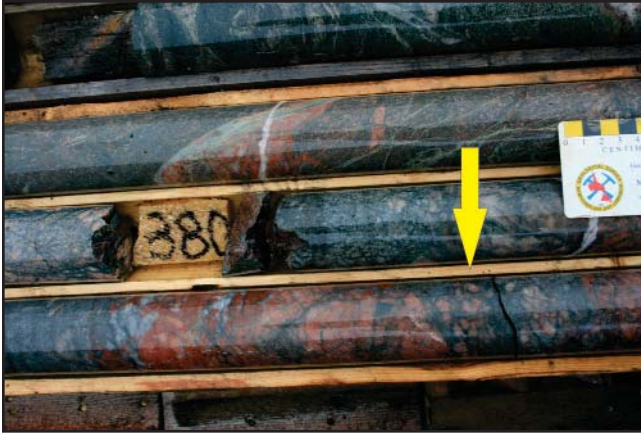
Plate 15. Feldspar-rich pegmatite overprinted by chlorite-rich brecciation; Two-Time deposit, DDH CMB-07-21, ~380 m depth.
