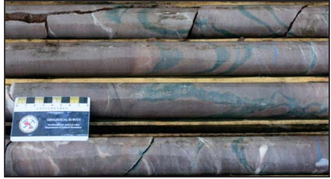
Plate 91. Oxidized sandstone overprinted by fractures displaying an influx of reduced fluids immediately above the mineralized zone of the Lower C Zone deposit (DDH ML-34, ~310 m depth).
