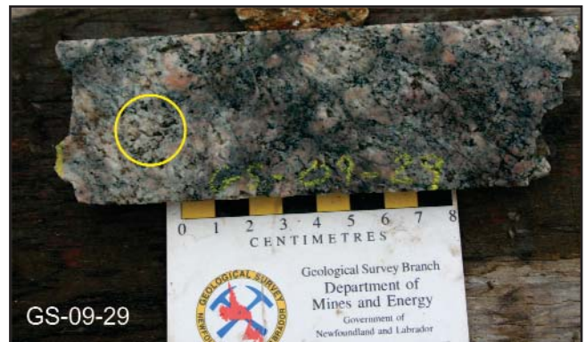
Plate 24. Hand sample displaying ‘vuggy’ textured zone, infilled with a pale-cream clay mineral (yellow circle) identified as phengitic illite on the basis of VIRS analysis.
