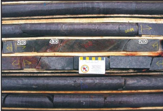
Plate 108. Anomalous radioactivity developed within brittle fractures in felsic volcanic rocks of the Sylvia Lake Formation, Madsen Lake Zone 4B prospect (DDH ML-MA-02, 20 m depth); white labels denote counts per second.
