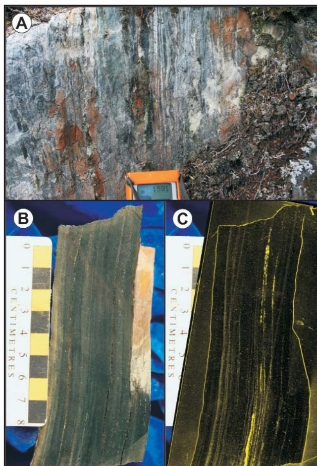
Plate 61. A. Uraniferous metasedimentary rocks with minor mafic tuff, Inda deposit, B. Mineralized metasedimentary rock displaying a strong foliation developed parallel to compositional layering within the sample, C. Autoradiograph of (B) outlining the roughly stratiform uranium mineralization (shown in yellow) within the sample.
