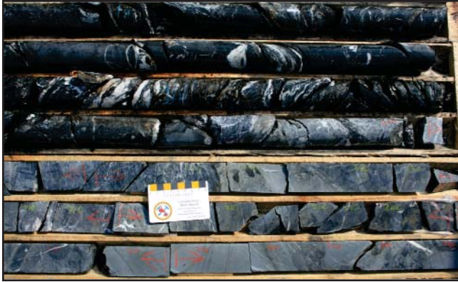
Plate 47. Mineralized and locally brecciated dolostone immediately overlain by sulphidic black shale hosting abundant quartz-carbonate veining; note mineralization is confined to the disrupted portions of the dolostone unit. Area 51 prospect, DDH MLA51-03, ~20 m depth.
