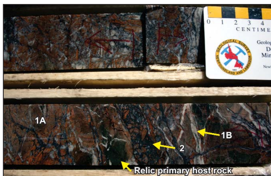
Plate 27. Early pinkish-orange hematite–albite alteration (Phase 1A) overprinted by white Fe-carbonate–quartz–albite alteration (Phase 1B), which is, in turn, cross-cut by dark-purple hematite-rich fracturing (Phase 2) and associated brecciation. Note pale-green patches of relatively unaltered mafic volcanic are still locally preserved. Moran Lake C Zone, DDH ML-3, ~55 m depth.
