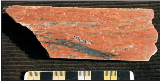
Plate 110. Quartz- and feldspar-phyric felsic metavolcanic rock displaying fracture-hosted magnetite alteration, Minisnakwa prospect.
