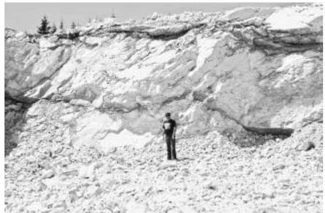
Plate 8. Coles Pond marble deposit showing quarry development face and stripped surface area.
