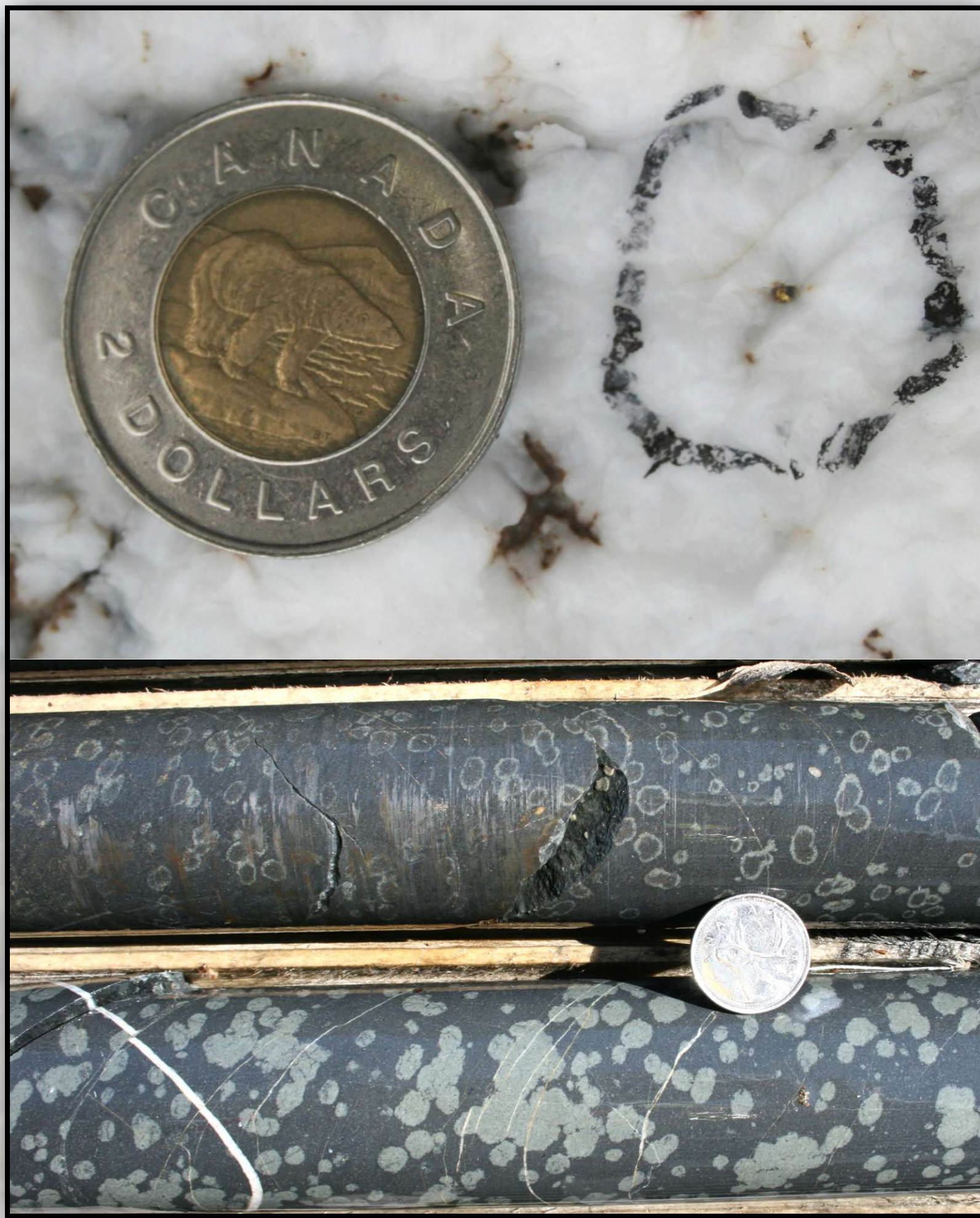
Top: Visible gold in crustiform quartz vein material Bottom: Unusual "spotty" alteration developed in spatial association with mineralized veins.
