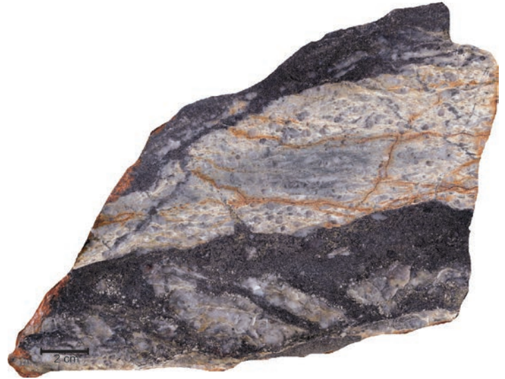
Polished slab exemplifying copper-lead-zinc mineralization; volcanogenic massive sulphide (VMS) occurrence.
