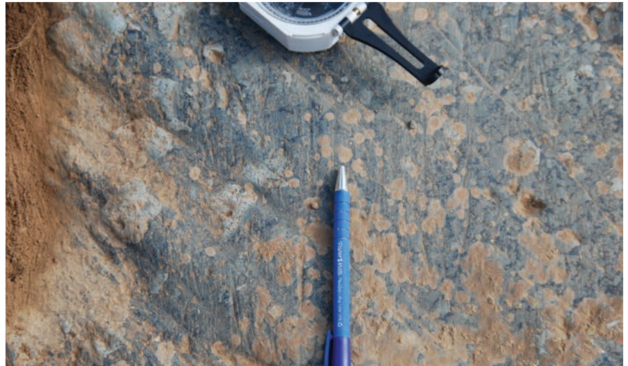
Erosional indicators (striae) in rock units north of the survey area. These indicators help reconstruct ice-flow histories. The smaller striae, indicated by the blue pen crosscut larger erosional features indicated by the compass. The depth and extent of the indicators can help define the most erosive glacial episode and thus help determine the dominant glacial-sediment transport direction.
