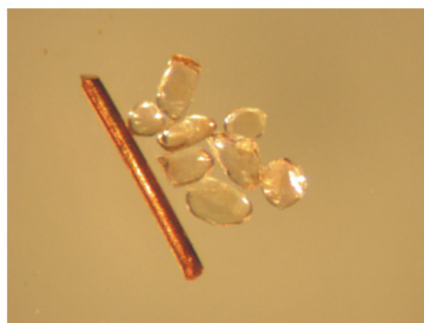
A graphic plot of U and Pb isotope data derived from analyses of zircons extracted from granite. The rock is 1348 million years old (1348.2 +/- 1.4 Ma). The lower picture shows the minute zircon crystals from which the age was obtained; the wire used for scale, is 0.1 mm in diameter.
