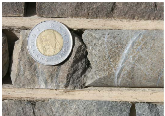
Quartz veining and sericite-quartz-sulphide alteration in drillcore, Hurricane prospect.
