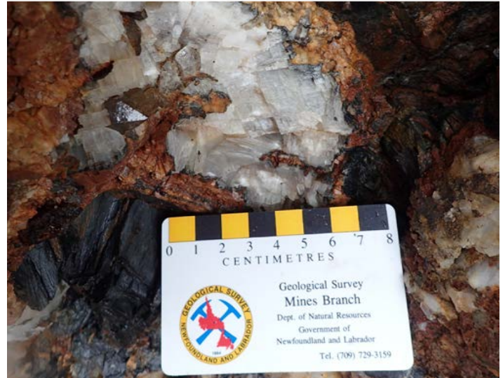
Carbonate-quartz vein surrounded by iron-rich alteration in shale/shales (?) at Pardy Head, close to Head of Bay d'Espoir.
