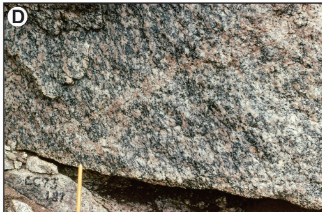
Plate 13.7. Pinware terrane foliated and gneissic quartz monzodiorite and K-feldspar megacrystic granitoid rocks. A. Lodge Bay quartz monzodiorite dated to be ca. 1590 Ma, discordantly intruded by metamorphosed mafic dyke (CG87-461), B. St. Augustin River megacrystic granitoid gneiss dated to be 1507 \pm 8 Ma (CG00-319), C. York Point megacrystic granitoid rock dated to be 1489 \pm 2 Ma, intruded by York Point mafic dykes (VN93-662), D. Pinware megacrystic granite 1466 \pm 8 Ma (CG93-187).
