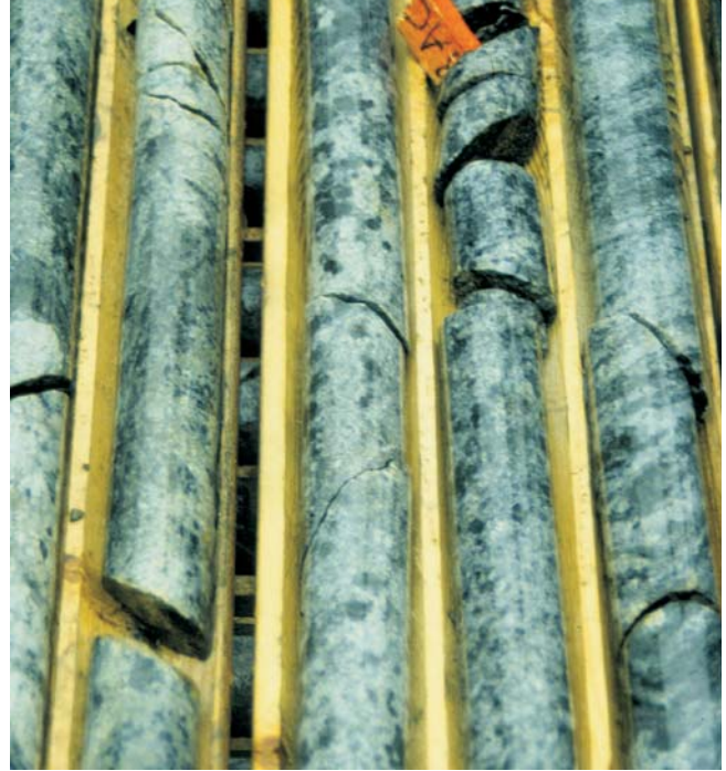
Plate 2. Typical intersection of ‘footwall gneiss’ below the base of the Pants Lake North intrusion. Most of this drillcore consists of white granitoid gneiss containing relict garnets (now partially retrogressed to cordierite); banded biotite-rich paragneiss visible at top right. Drillcore is approximately 4 cm in diameter.
