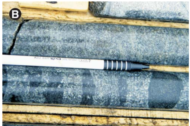
Plate 10. A. Typical fine- to medium-grained olivine gabbro from the South intrusion; upper sample shows a typical ‘speckly’ plagioclase–porphyritic variety, scale in cm. B. Drillcore from fine- to medium-grained gabbro of the South intrusion. The upper part of the picture shows subtle colour variations indicative of variations in mafic mineral content due to magmatic layering. The dark patches in the lower part of the picture are inclusions of melagabbro, probably derived from disrupted cumulate units.
