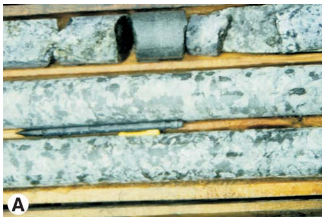
Plate 33. A. Granitoid gneiss from just below the basal contact of the North intrusion; the grey patches were originally garnets, but have now been entirely retrogressed to cordierite due to contact metamorphism. B. Assorted footwall gneiss rock types, including banded pelite paragneisses at top, pink granitoid gneiss in the centre, and migmatitic paragneiss at the bottom. Note the copper-rich sulphide vein in the lower sample, which resembles the high-grade zone intersected in hole SVB-97-75. Drillcore approximately 4 cm wide.
