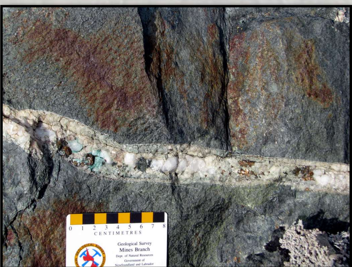
Chalcopyrite-bornite-malachite hosted within quartz + carbonate vein, cutting fine-grained gabbro sill. (MODS occurrence 13K/05/Cu003)
