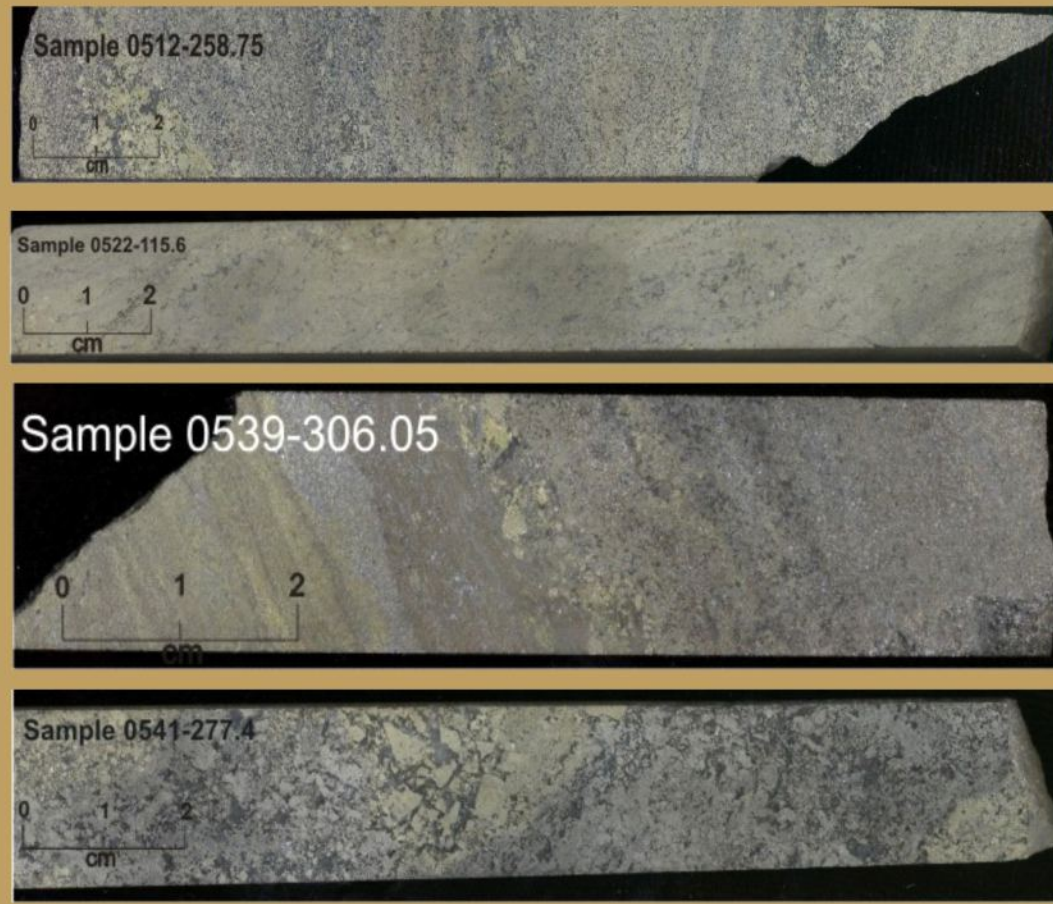
Figure 3.a. Photograph of polished slab consisting of fine-grained brown sphalerite and silvery grey galena interbedded with fine- to medium-grained pyrite with pyrite porphyroblasts hosted in silica +/- carbonate gangue. Sample 0512-258.75. Note: Labeling stands for DDH (0539) sampled at a depth of 306.05m.
