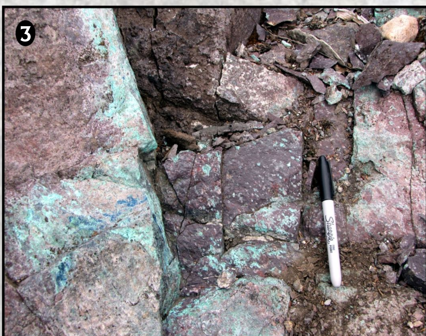
3 Malachite and azurite staining and disseminated chalcocite in strongly hematized, amygdaloidal basalt flow. Mineralization occurs as amygdules and as fine-grained aggregates along fracture surfaces. (Salmon Lake Formation, south shore of Seal Lake, Ellis Pond Occurrence No. 75, MODS No. 13K/05/Cu028).
