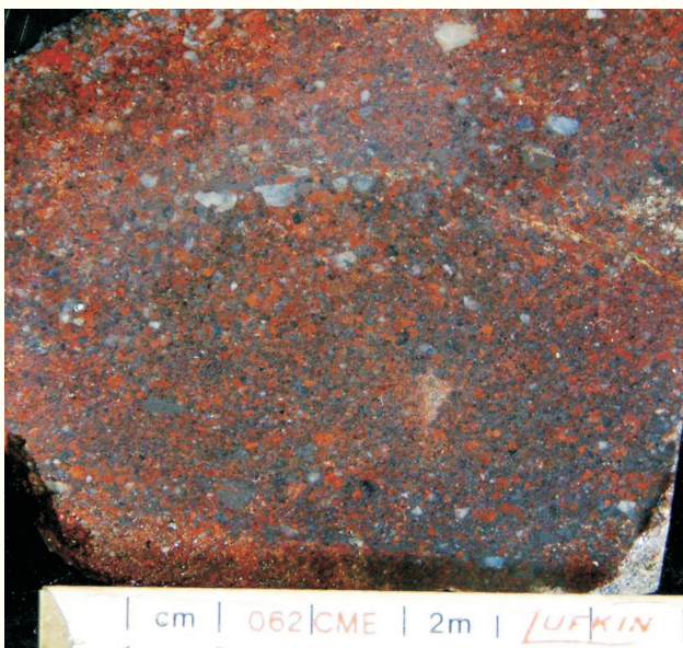
Figure 13. High-grade sandstone float from the Deer Lake Basin grading 10.2% U 3 O 8 and 529 g/t Ag (photo courtesy of Altius).
