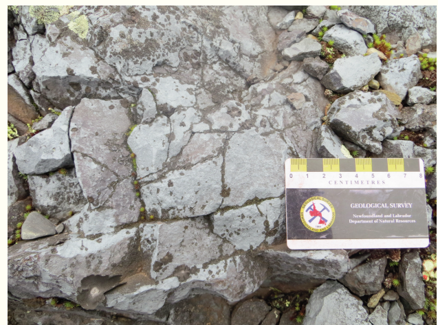
Figure 10. Hard, blue hematite-rich DSO ore from the Sawyer Lake deposit (Labrador Iron Mines).
