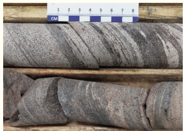
Figure 5. Banded metataconite ore from the Julienne Lake deposit, displaying coarse-grained specular hematite.
