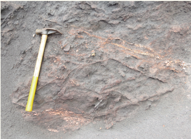
Figure 9. Soft, friable DSO ore cut by leached silica veins from Timmins No. 4 deposit (Tata Steel Minerals Canada/New Millennium Iron Corp.).
