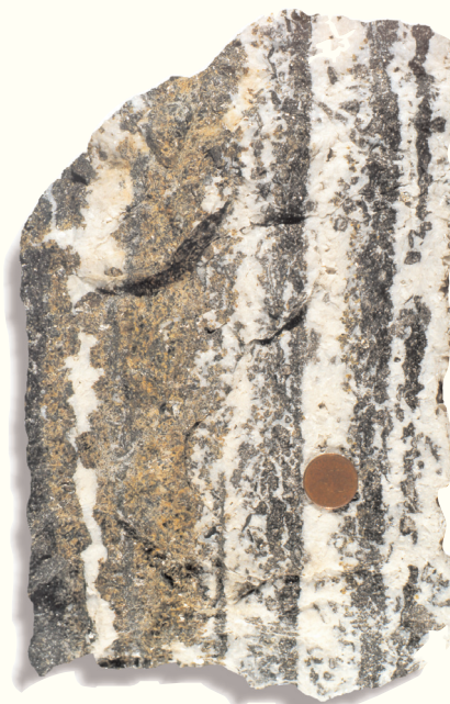
Figure 4. Daniel's Harbour ore. Early, grey, burrowed dolostone has been replaced by yellow sphalerite and white dolomite, locally enclosing suspended fragments of dolostone in pseudobreccia texture.
