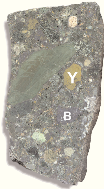
Figure 7. Buchans transported-ore breccia. Note clasts of massive chalcopyrite yellow ore (Y) and sphalerite–galena black ore (B)
