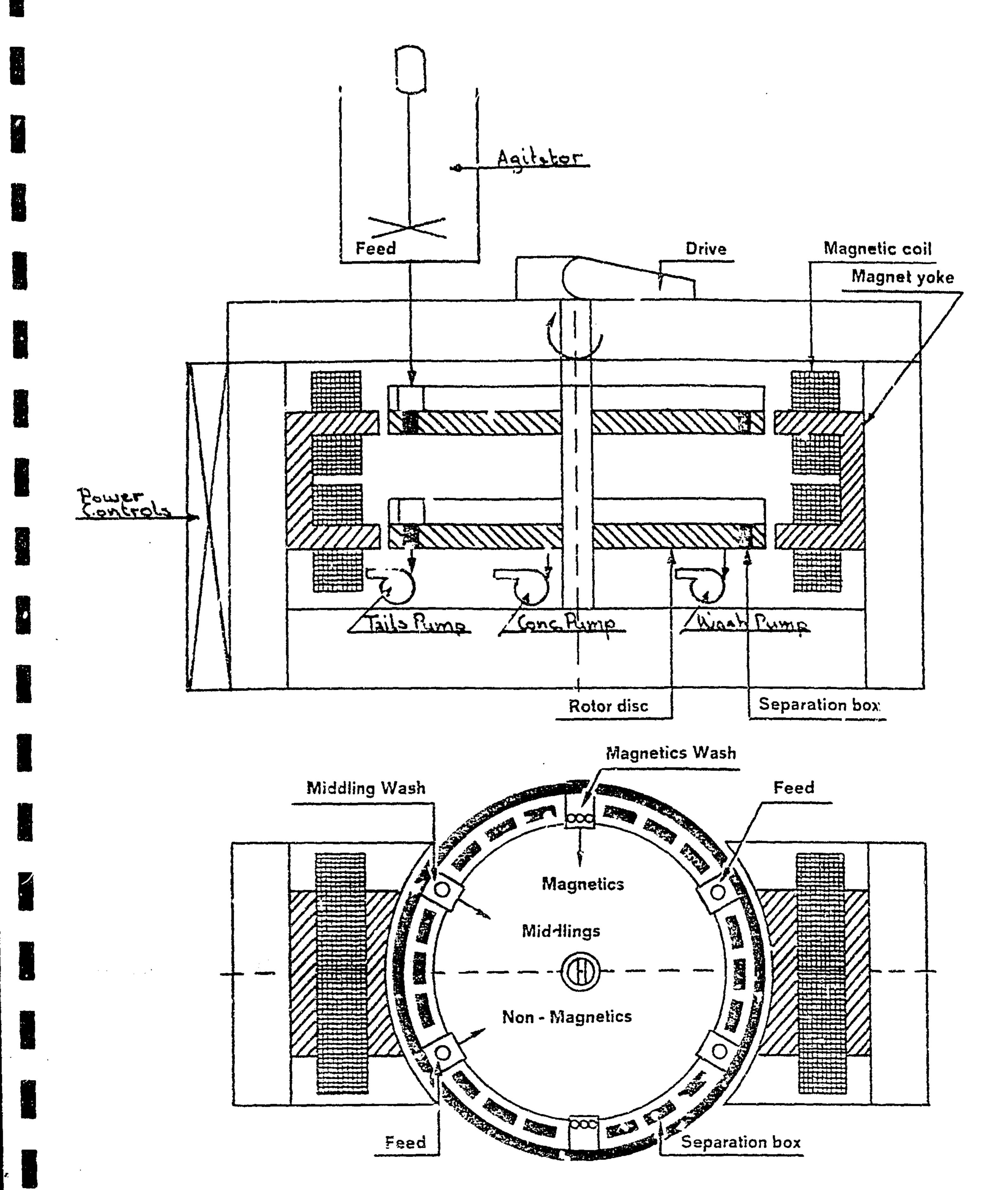
Fig. 1 Operating principle of the Humboldt manufactured
