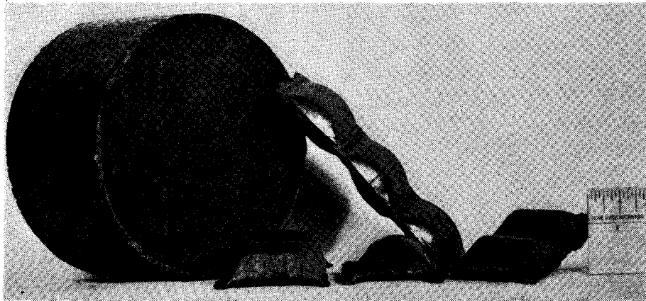
Fig. 17 — Various types of briquette produced from SL sponge iron.
