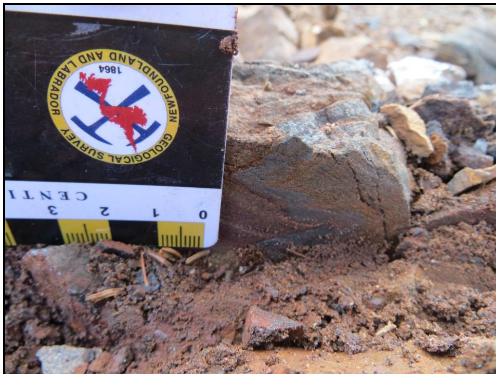
Figure 16: Tight isoclinal folding of specularite band (from Trench 1, close to collar of JL-10-11A)
