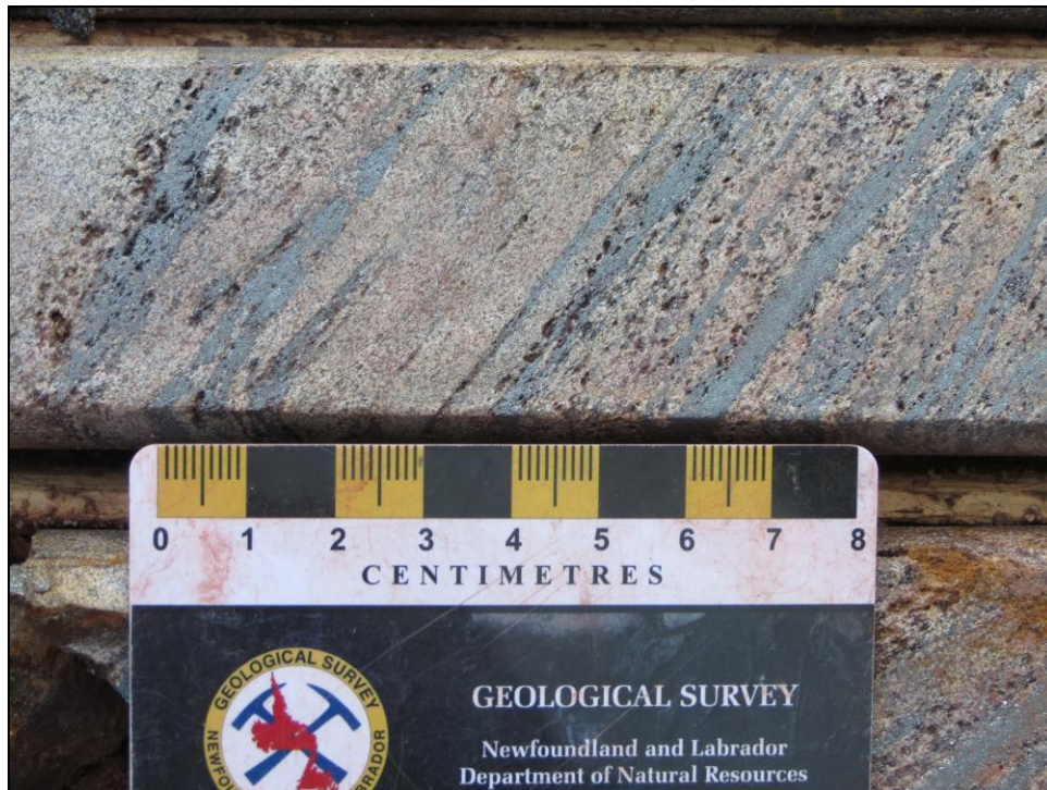
Figure 5: Banded QS iron formation, with quartz-rich layers and bands of pure specularite (from JL10-16)
