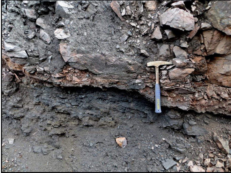
Figure 8: Gently dipping bed of Mn-rich iron formation, from north end of Trench 1
