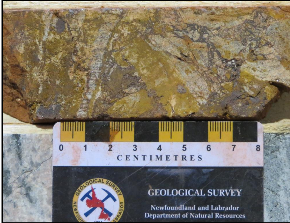
Figure 11: Brecciated and strongly altered Lower Iron Formation (from JL10-14)
