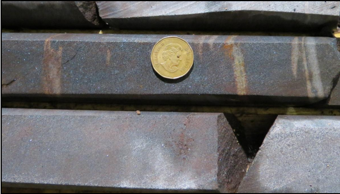
Figure 4: Massive QS iron formation with thin quartz-rich layers (from JL10-15)
