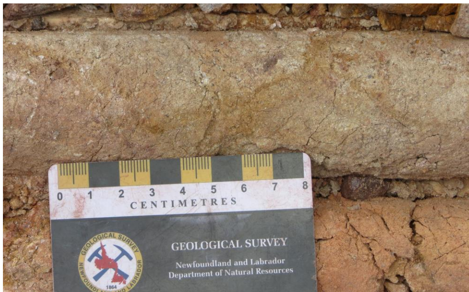
Figure 13: Intensely leached micaceous sand in the Wishart Quartzite (from JL10-17B)
