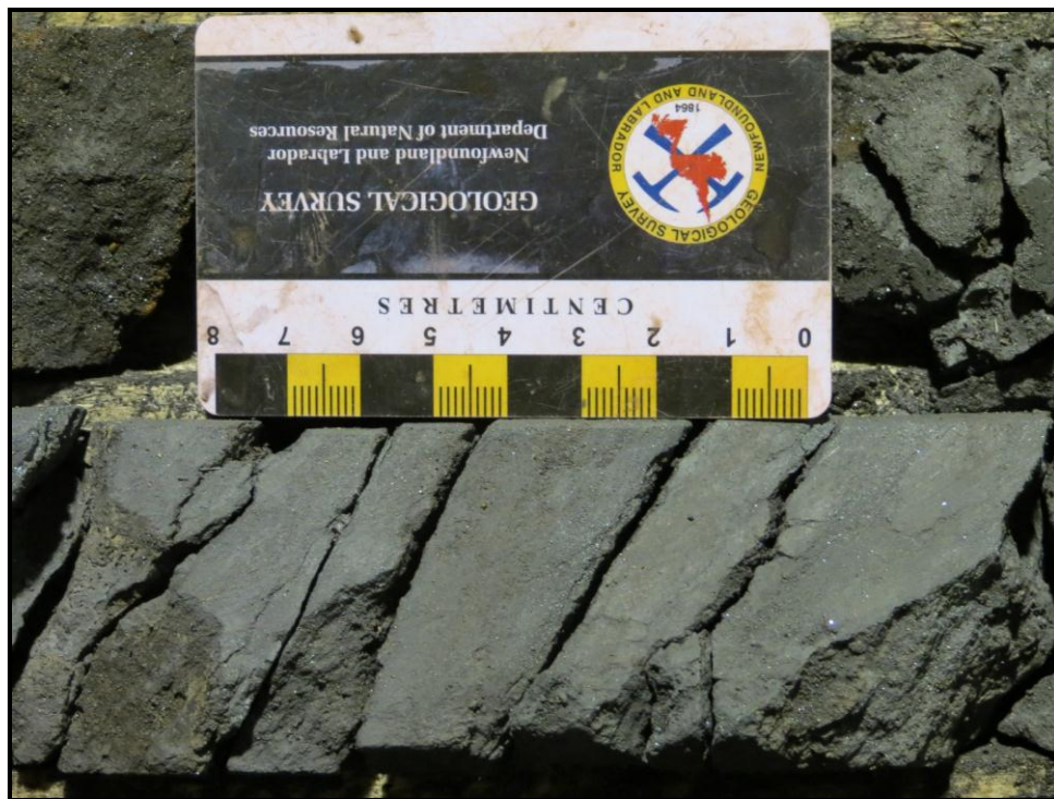
Figure 7: Pyrolusite-bearing, Mn-rich iron formation, with typical black sooty appearance (from JL10-17B)
