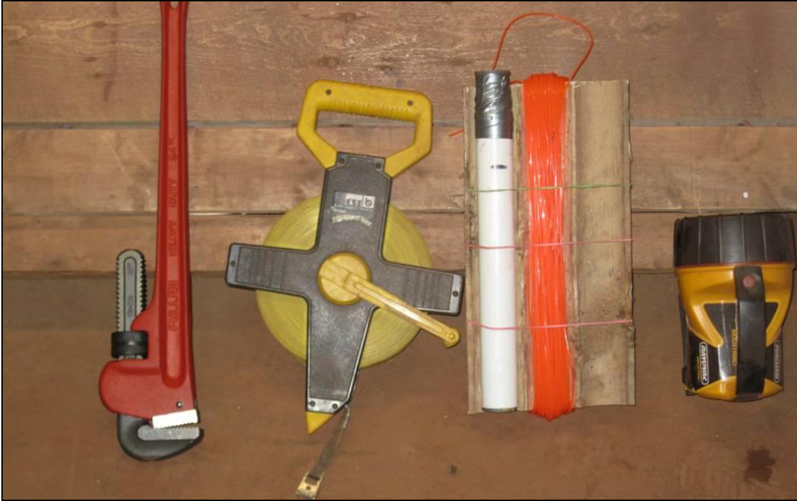
Photo 12: Water depth sounding apparatus.
