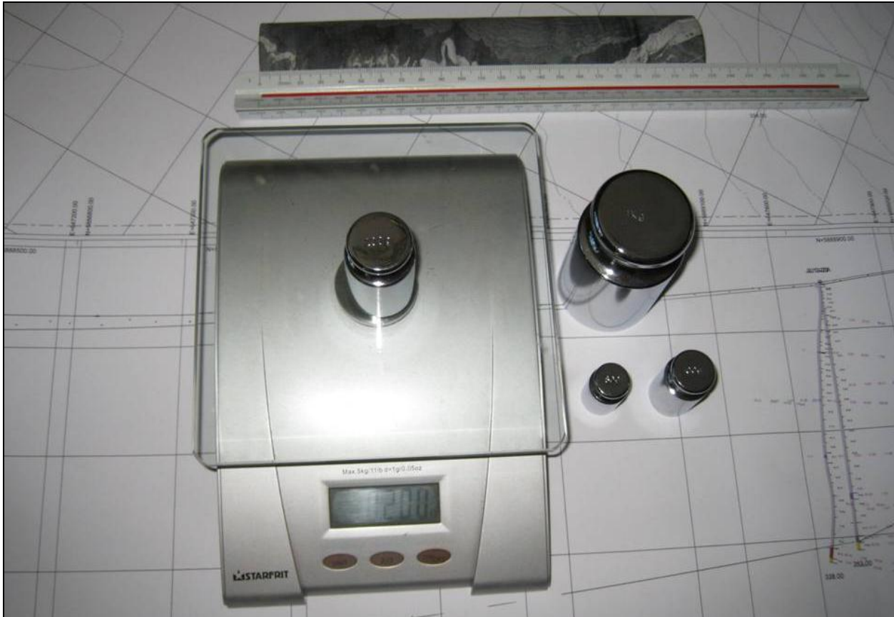
Photo 3: Dry bulk density measuring apparatus.
