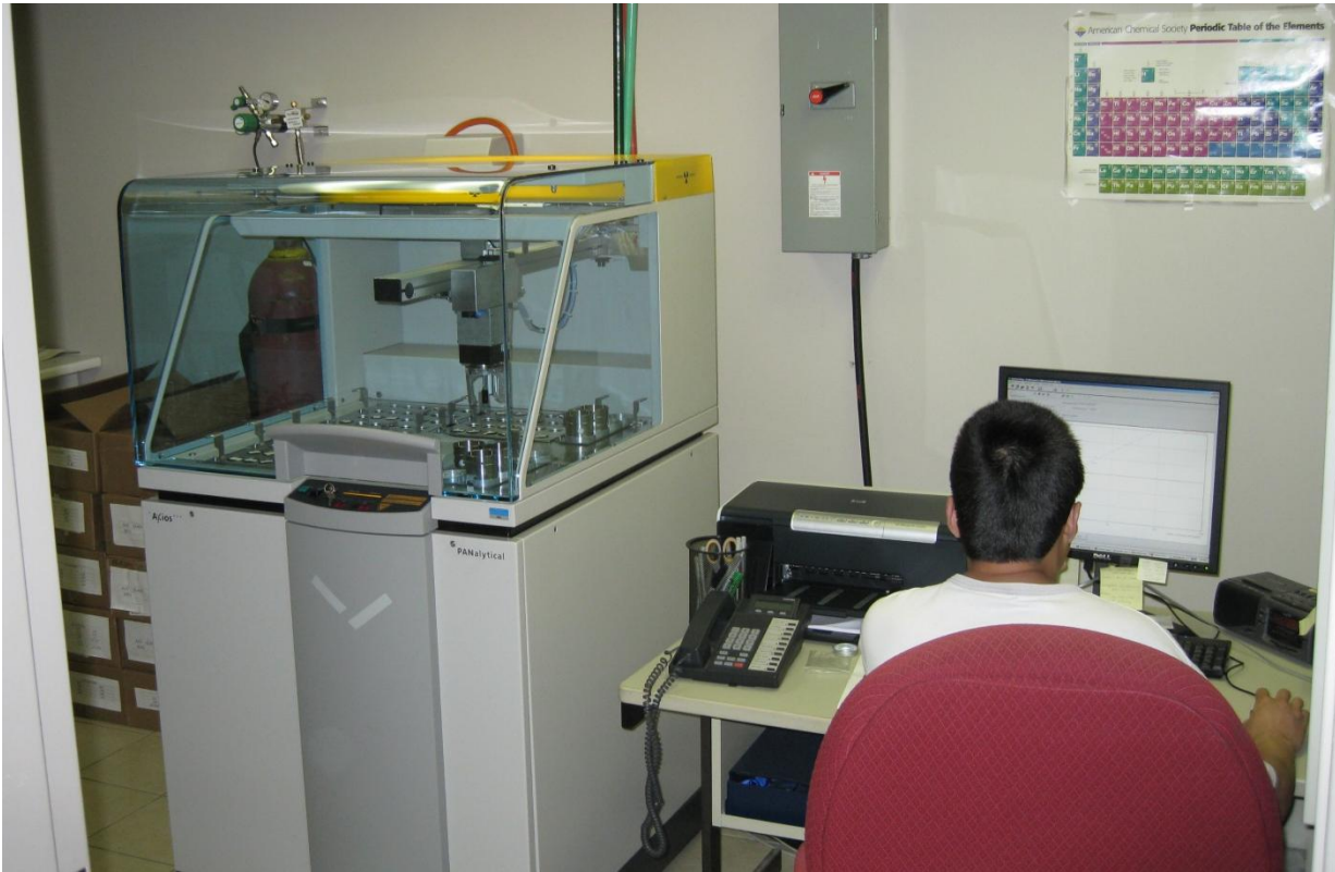
Photo 2: Actlabs Panalytical Axios Advanced wavelength dispersive XRF
