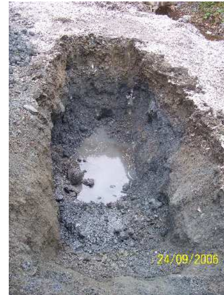
Photo 44: Petroleum Hydrocarbon Sheen – Test Pit NC-TP23.
