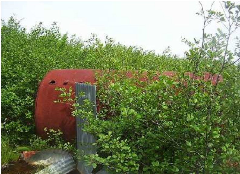
Photo 13: Discarded Fuel Tank – Possible UST. (Former Equipment Parking Area)
