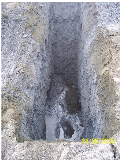
Photo 13: Asbestos Fibres within Test Pit WR-TP3. (Former Pit Office Area)
