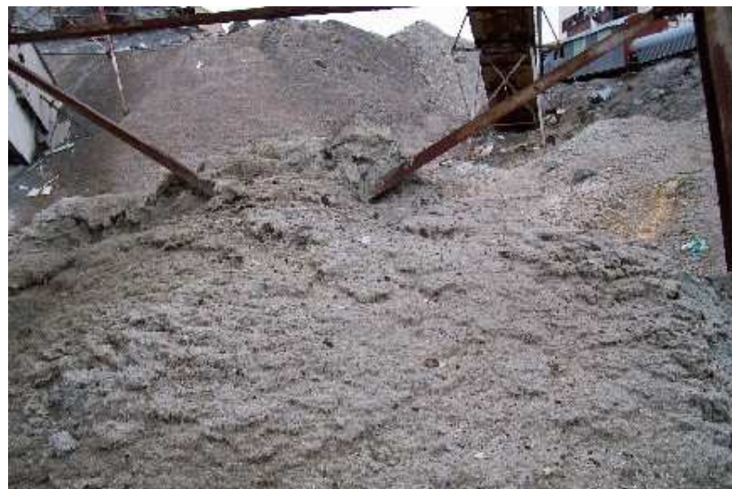
Photo 18: Exposed Friable Asbestos – Between Dry Rock Storage Facility and Secondary Crusher Building.
