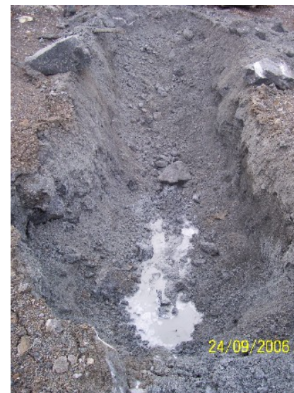
Photo 14: Asbestos Fibres within Test Pit WR-TP4. (Former Pit Office Area)
