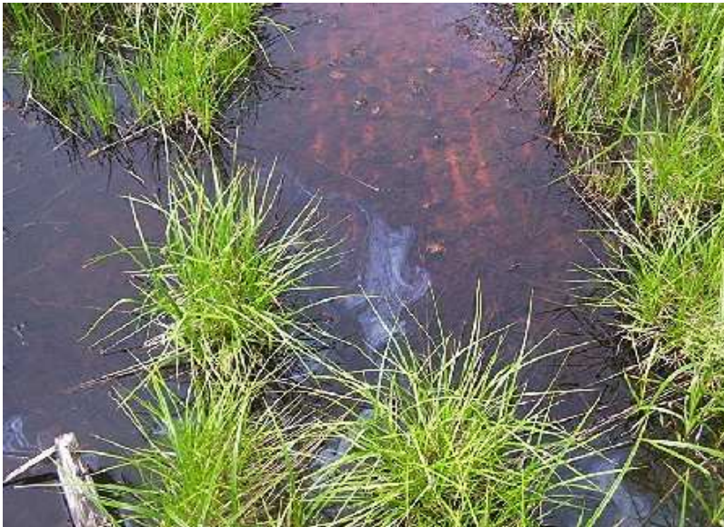
Photo 15: Petroleum Hydrocarbon Sheen. (Former Equipment Parking Area)
