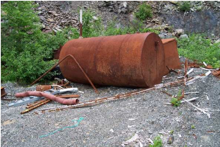
Photograph 11. Discarded 10,000-Gallon UST (Equipment Storage Area)
