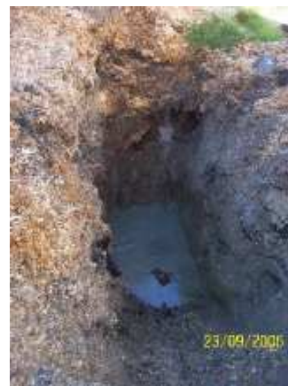
Photo 20: Petroleum Hydrocarbon Sheen – Test Pit ML-TP18. (Southwest of the Power Centre)
