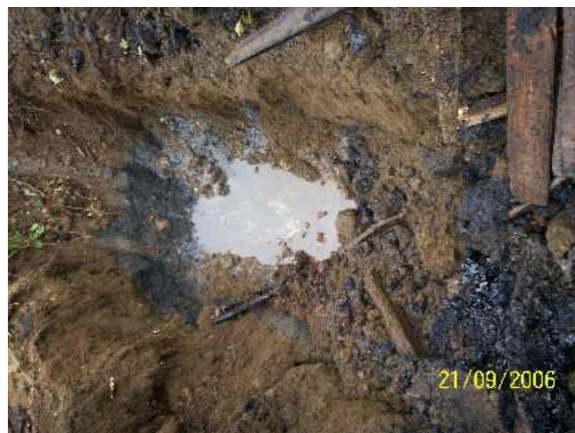
Photo 18: Test Pit WH-TP11 - Petroleum Hydrocarbon Sheen.
