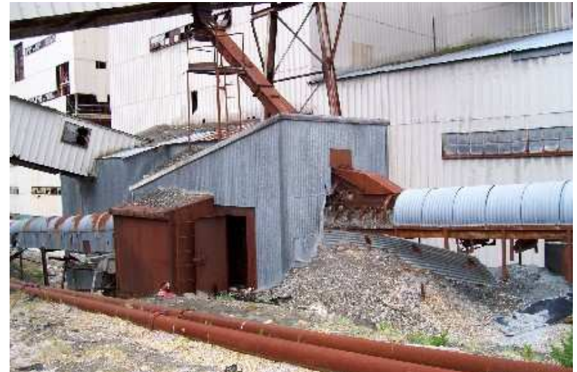
Photo 16: Exposed Friable Asbestos – Conveyor on Northside of Secondary Crusher Building.
