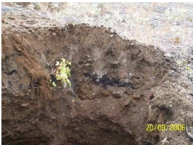
Photo 17: Test Pit WH-TP6 - Layer of Bunker C. (0.3 m to 0.4 m bgs)
