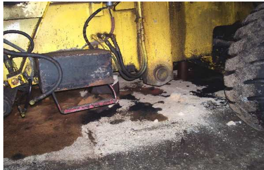
Photo 36: Staining Underneath Equipment Along Floor Drains – Former E&R Building.
