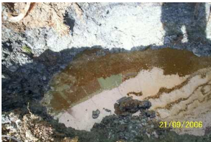
Photo 19: Free Product – Test Pit ML-TP3. (Southside of Dry Mill Building)
