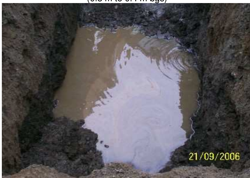
Photo 19: Test Pit WH-TP12 - Petroleum Hydrocarbon Sheen.
