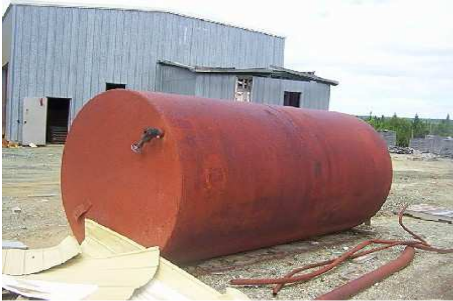
Photo 5: Possible Discarded UST - South of Maintenance Garage. (Rambler Main Mine)
