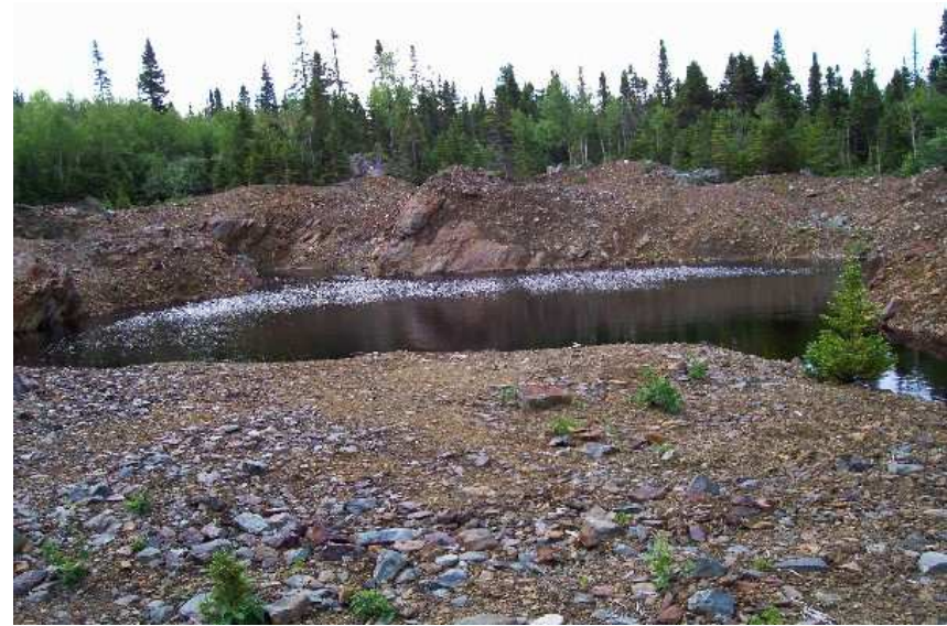
Photo 2: Open Pit – Filled with Water. (Note the Potential Acid Generating Waste Rock)
