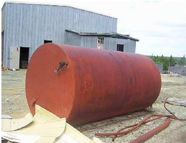
Photo 35: Discarded 5000-Gallon UST.
