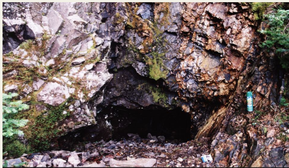
MacKay Vein and Adit Portal (Can for scale), 12.4 g/t assay Au taken from 15 cm wide chip sample from above the middle of adit
