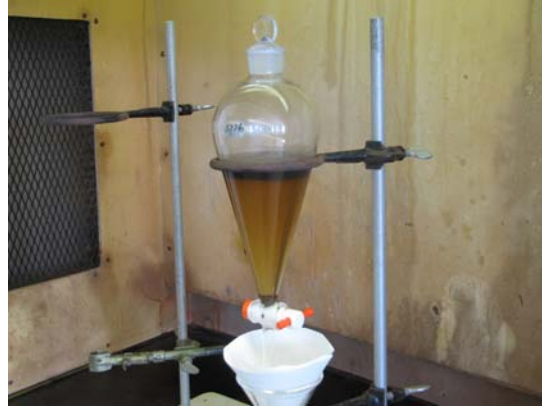
Figure 13: Heavy-liquid separation of a panned concentrate. The lighter minerals can be seen floating in the tetrabromoethane separating medium which has a specific gravity of 2.97. The heavy minerals are drawn off at the bottom, filtered and washed.
