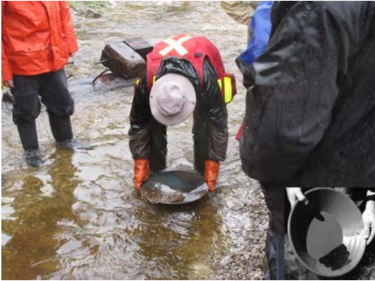
Figure 12: Panning stream gravels. In the larger photograph, a conical “Batea” pan is being used. The inset shows a typical panned concentrate in a flat-bottomed pan. This can be analyzed in its entirety, panned further, or subjected to heavy-liquid separation.
