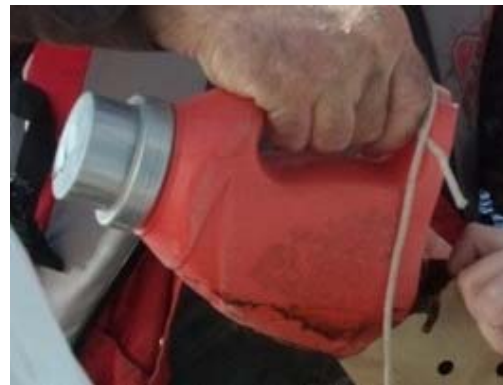
Figure 11: Plastic sample scoop. The cap can also be removed to enable pouring off excess water.
