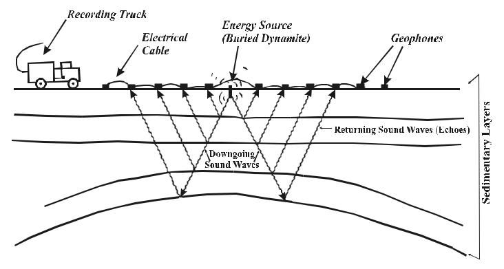
**Figure 6.5 - Seismic Exploration**
