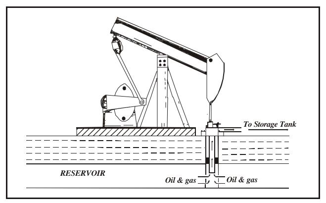
Figure 10.3 - Artificial Lift
