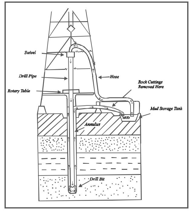
Figure 8.5 - Circulation Path of Drilling Mud
