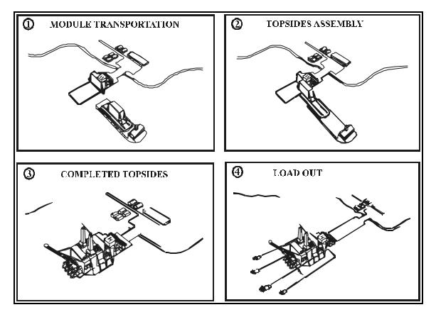
**Figure 12.2 - Assembly Sequence for Topsides Facilities**
