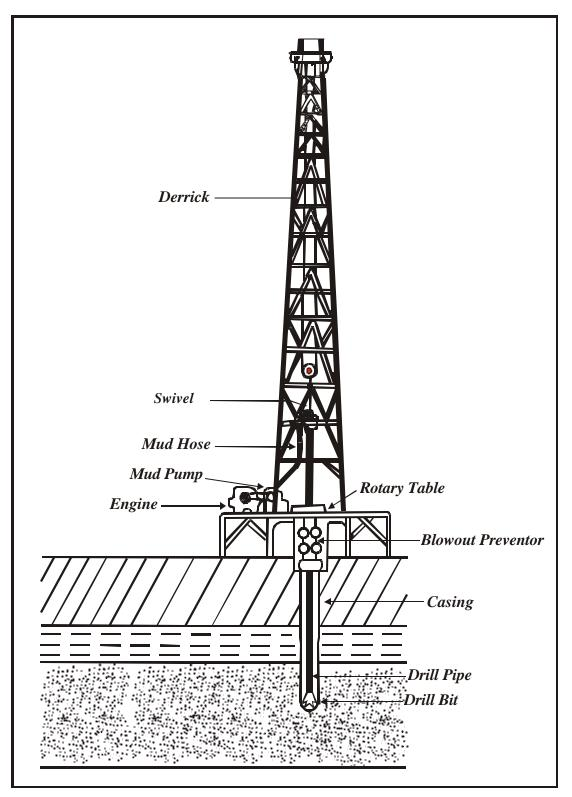
Figure 8.4 -Drilling Rig
