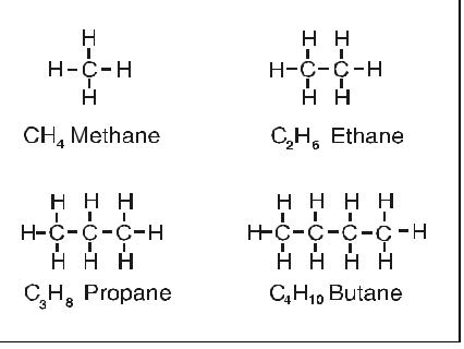
Figure 1.1 - Hydrocarbon Molecules
