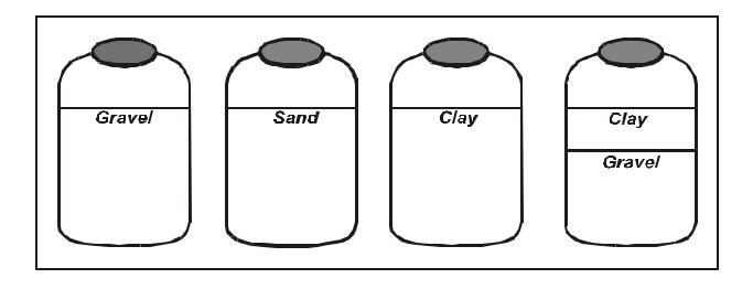
Using the measuring cup add water to each until no more will soak in and it just covers the surface. Record the volume added in each case.
