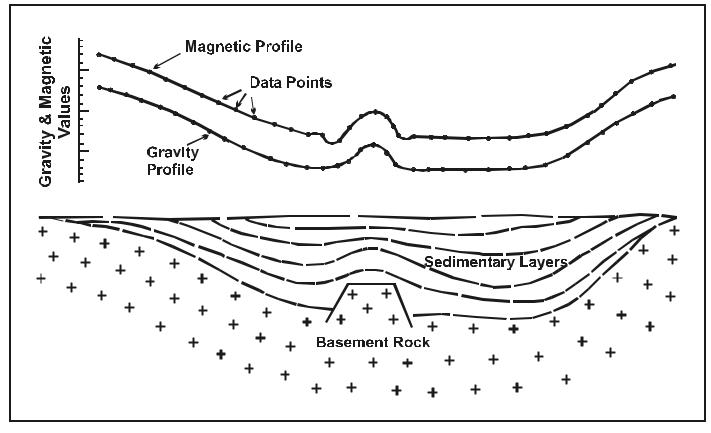
Figure 6.3 - Gravity and Magnetic Profiles
