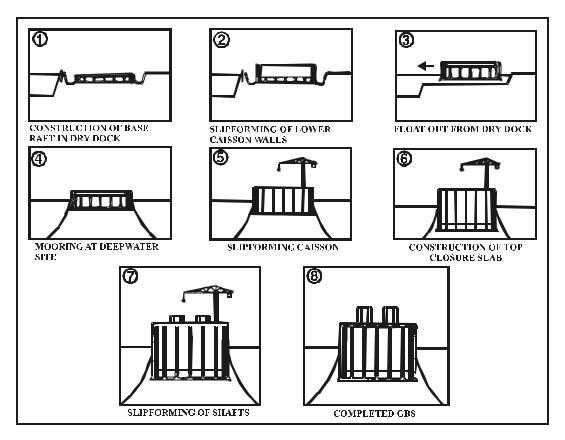
Figure 12.1 - Construction Sequence for GBS
