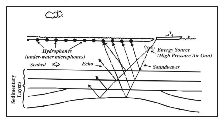
Figure 6.7 - Offshore Seismic Exploration
