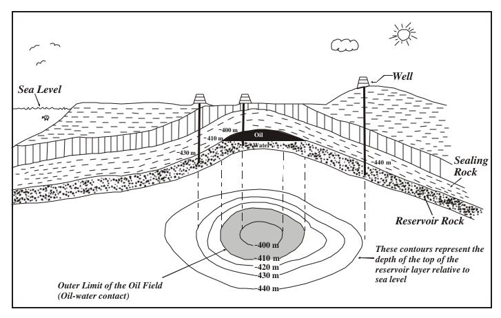
Figure 5.1 - Subsurface Structure Contour Map
