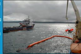
Standard Offshore SVSS skimming system being deployed from supply vessel.
