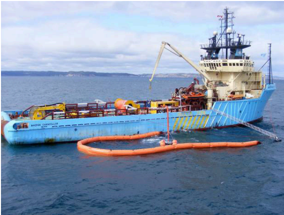
Single Vessel Side Sweep (SVSS) System (Synergy 2009)
