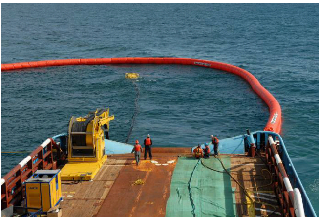
Transrec 150 Skimmer in Apex of NorLense 1200-R Boom (Synergy 2009)
