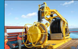
Tranrec 150 skimmer ready for deployment from the deck of a supply vessel
