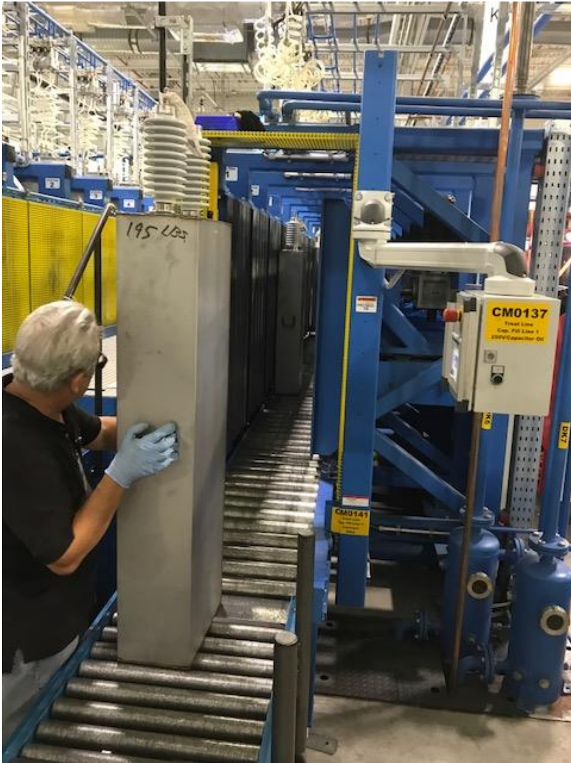
Photo 5: Drying and oil filling steps.
