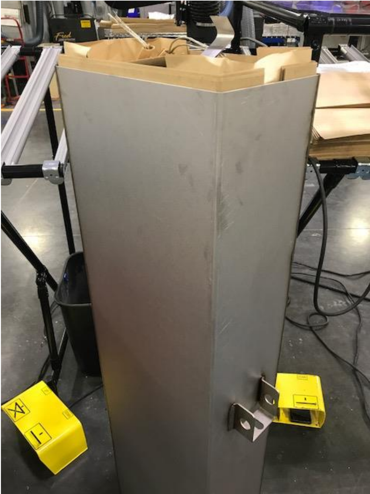
Photo 3: Capacitor inserted into the capacitor can.
