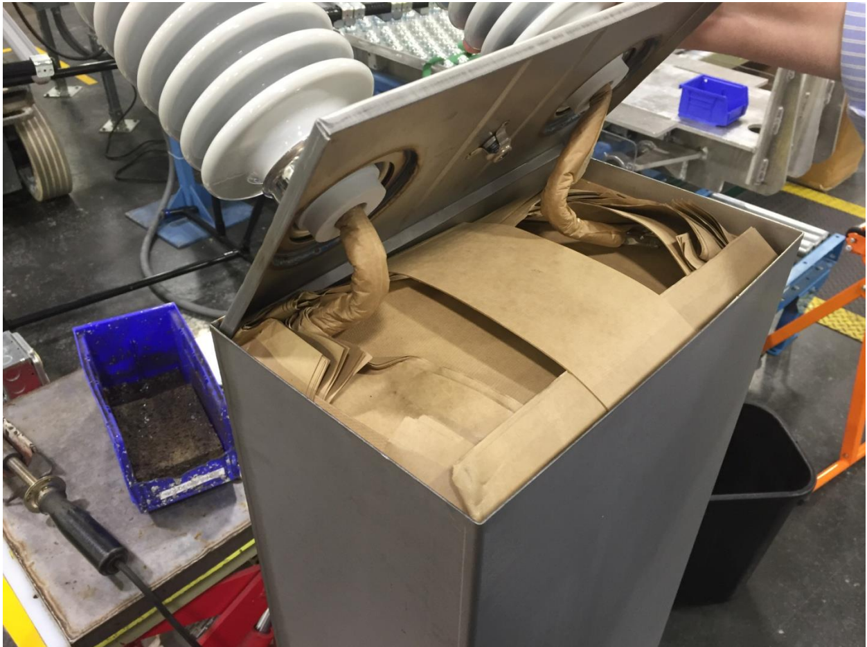
Photo 4: Final assembly prior to lid welding.
