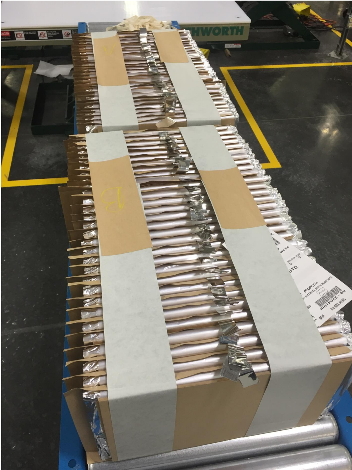
Photo 2: Capacitor bundles with connector tabs ready for assembly.
