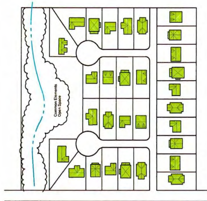
Single Family Detached Cluster Development - 10 acres - 30 lots - 7,000 sf Minimum Lot Size - Minimum Open Space/Common Elements - 15% of Total Tract
