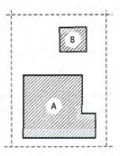
**LOT FRONTAGE** means the horizontal distance between side lot lines measured at the building line (the distance between points **A** and **B** in illustration at right).
