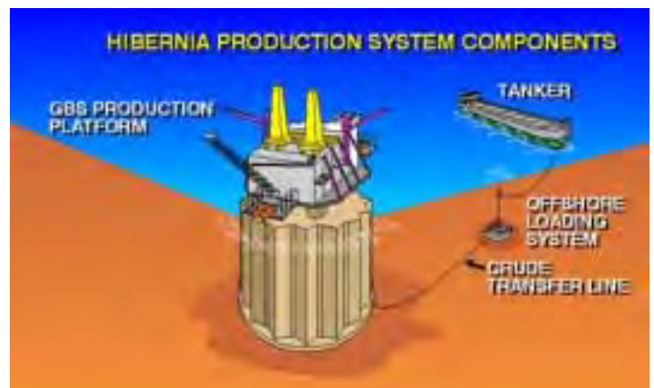
Hibernia Production System Components
