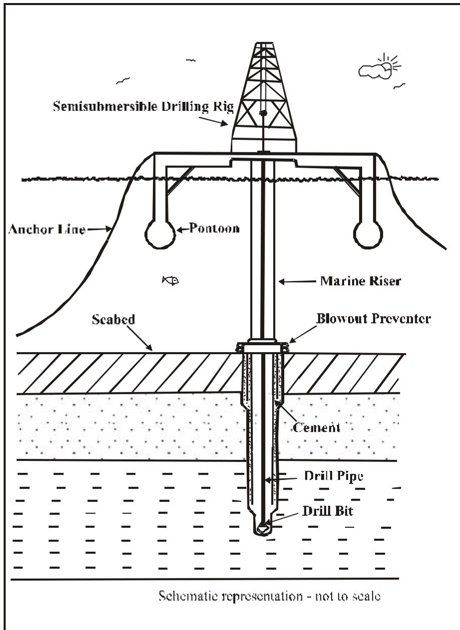
**Figure 9.2 -Semisubmersible Drilling Rig**
