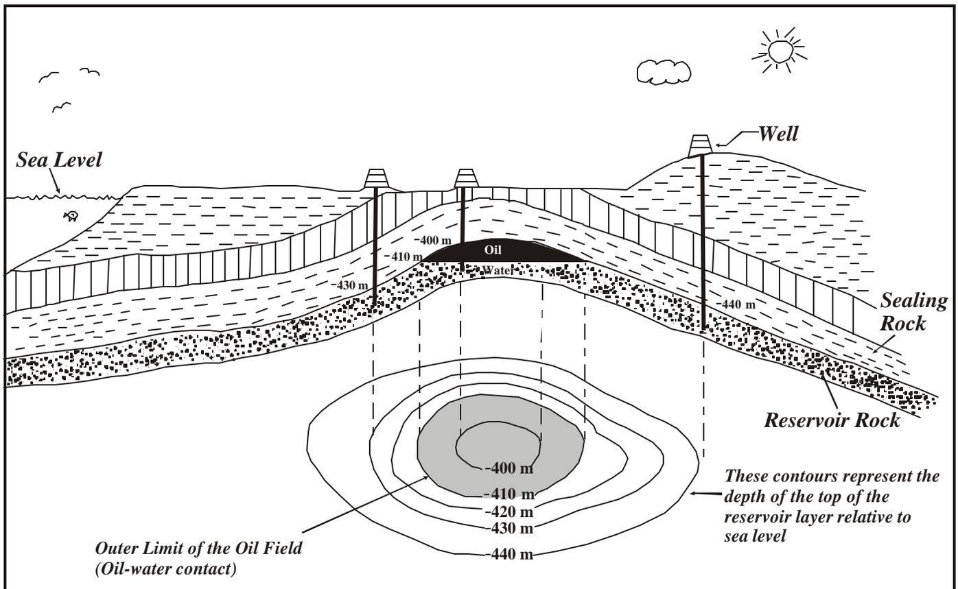
Figure 5.1 - Subsurface Structure Contour Map
