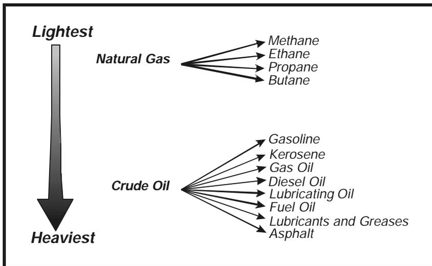
**Figure 1.2 - Petroleum and some of its components**
