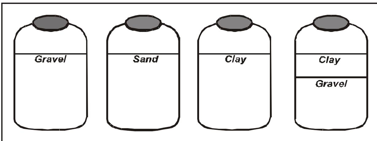
Using the measuring cup add water to each until no more will soak in and it just covers the surface. Record the volume added in each case.
