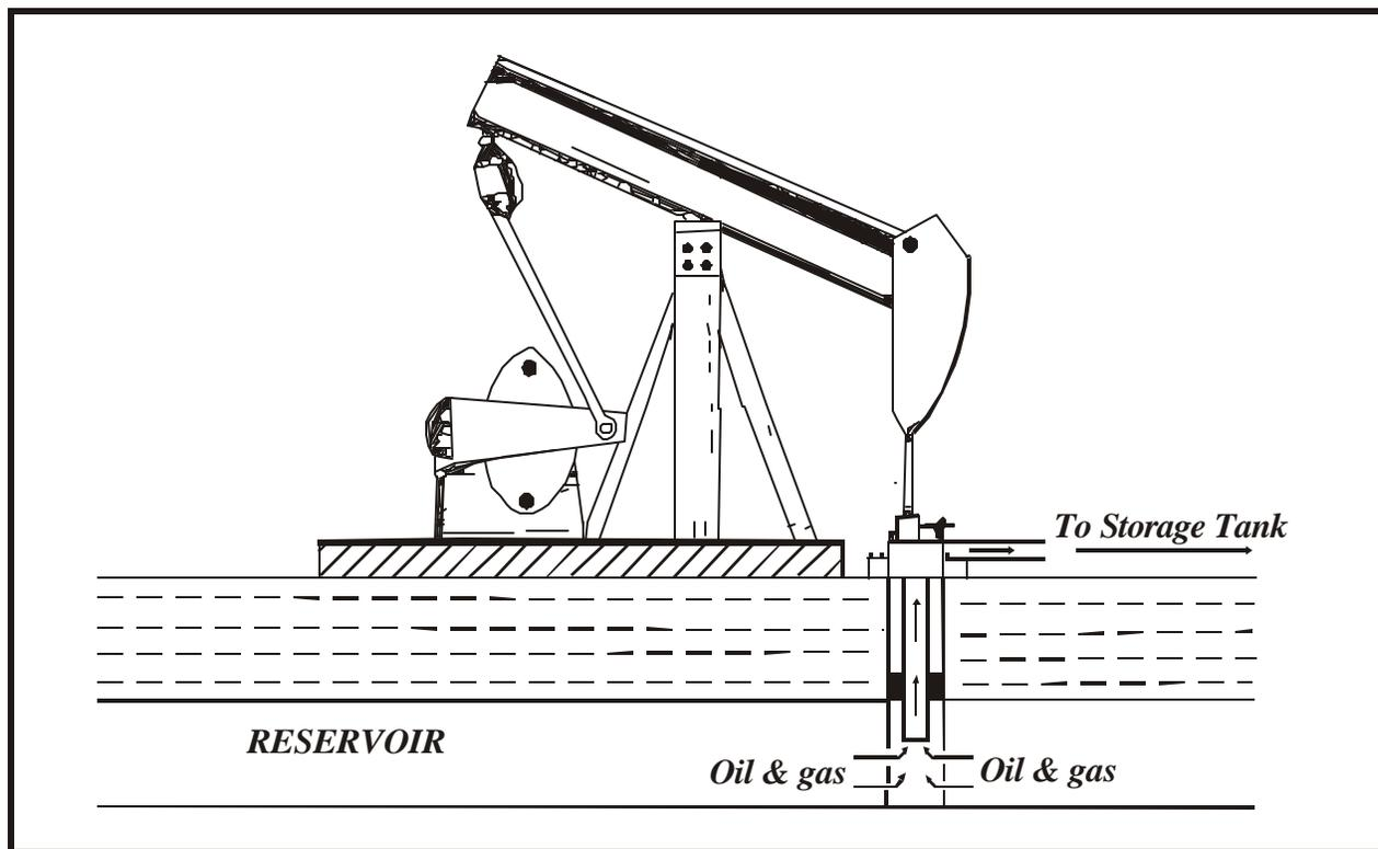
Figure 10.3 -Artificial Lift
