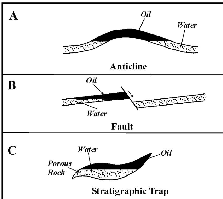
**Figure 4.2 - Hydrocarbon Traps**
