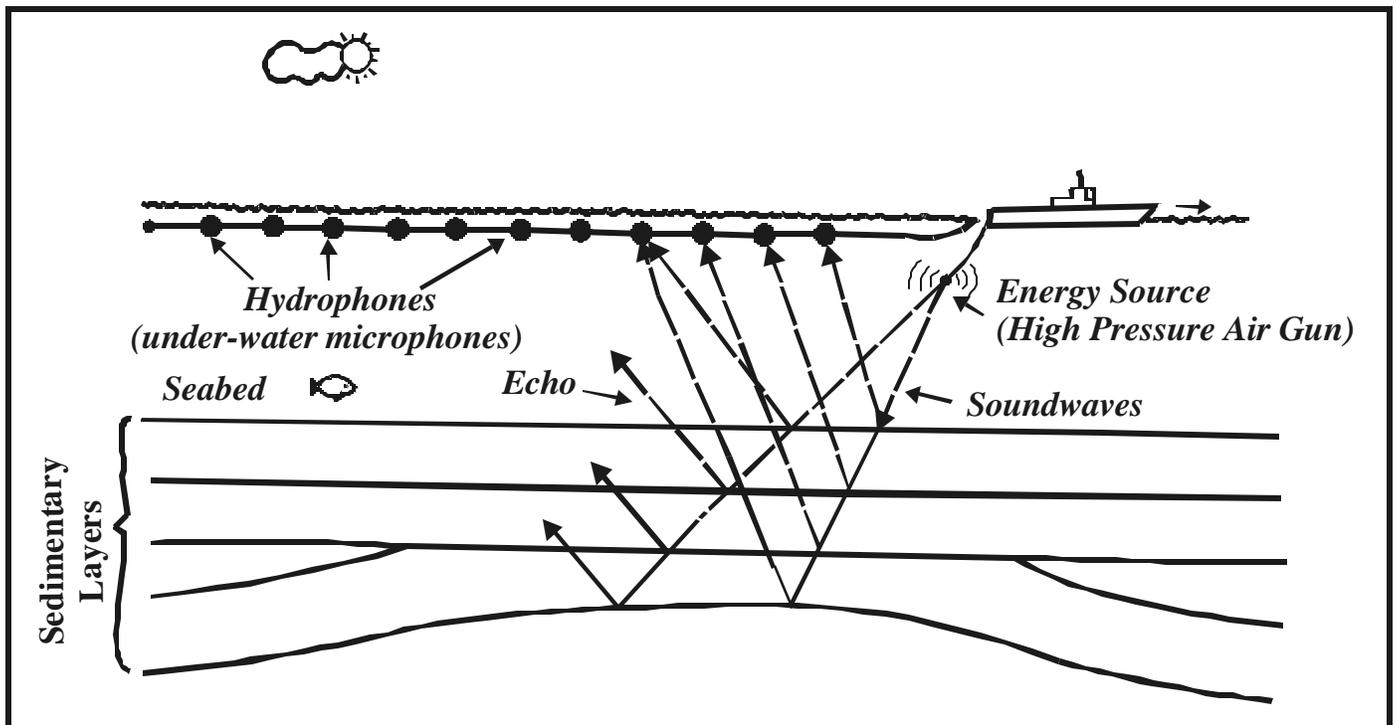
Figure 6.7 - Offshore Seismic Exploration
