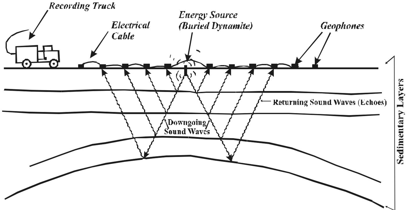
**Figure 6.5 - Seismic Exploration**
