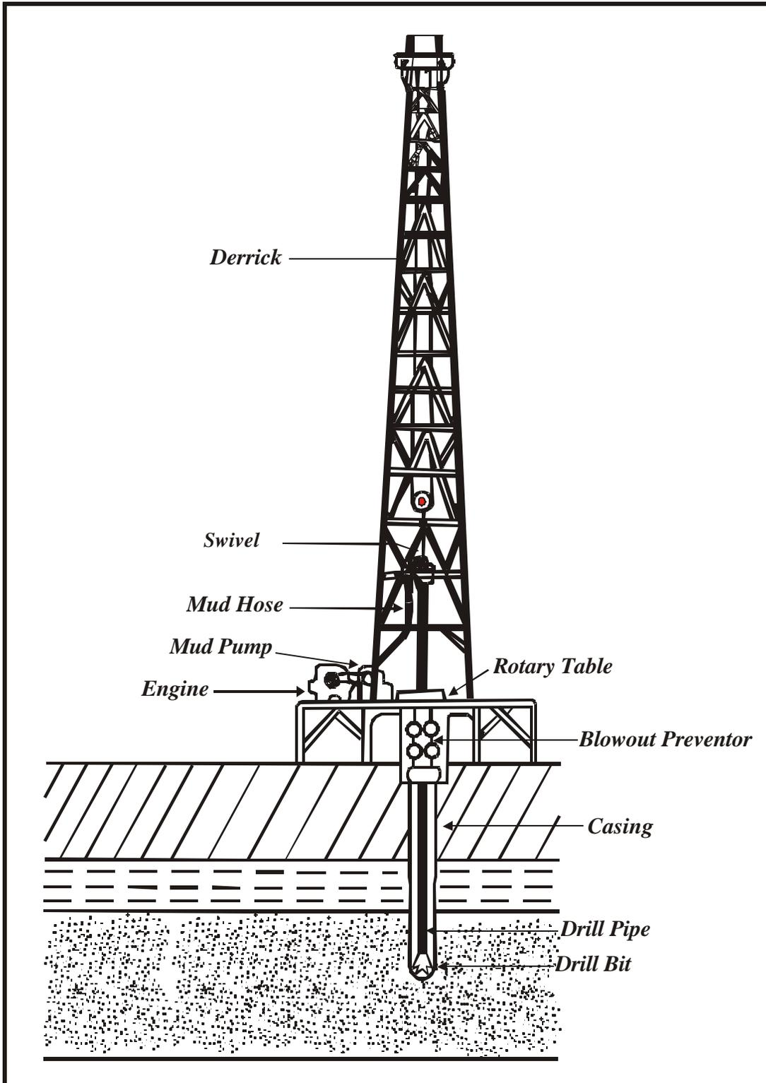
**Figure 8.4 -Drilling Rig**
