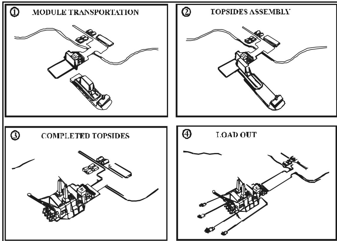
**Figure 12.2 - Assembly Sequence for Topsides Facilities**
