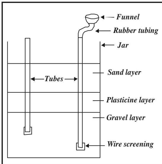
Place the tubes in the jar as shown in the diagram. Pack gravel into the bottom half of the jar around the tubes. Firmly pack a layer of plasticine on top of the gravel and seal tightly around both the tubes and the edge of the jar. Fill up the rest of the jar with sand.
