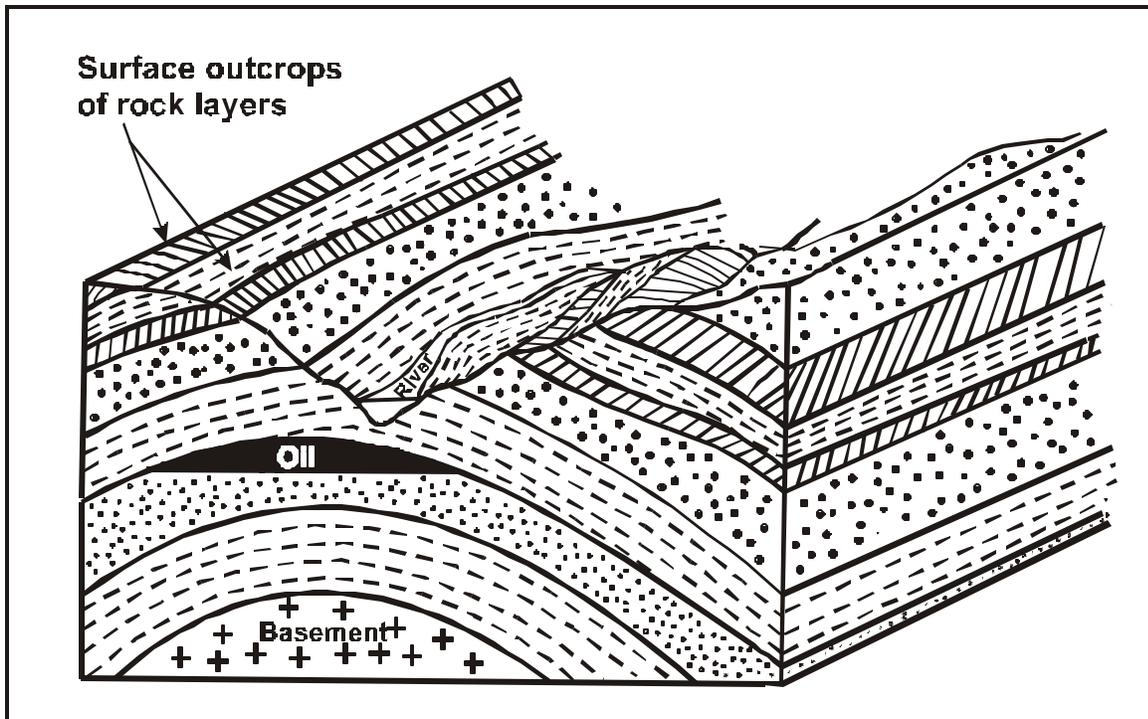
**Figure 6.1 - Eroded Anticline**
