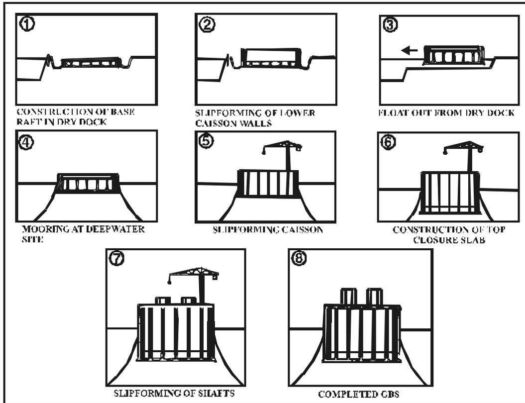
**Figure 12.1 - Construction Sequence for GBS**
