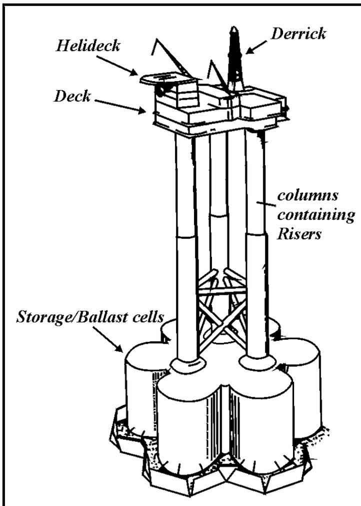
**Figure 10.5 - Gravity Base Structure Production Platform**
