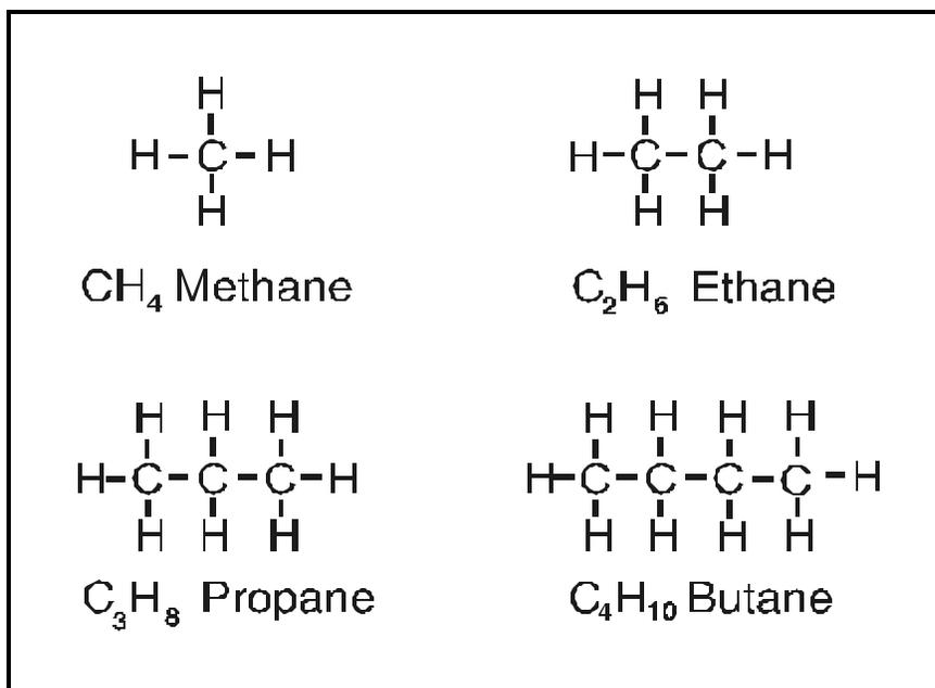
**Figure 1.1 - Hydrocarbon Molecules**
