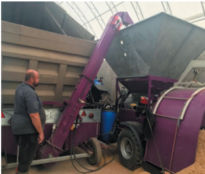
Processing high-moisture wheat with the Murska bioprocessor. Grain is offloaded from a dump truck into a 'fill device' that augers it into the Murska hopper where it is first rolled, then inoculated, and finally extruded to be loaded into a bunker silo.
