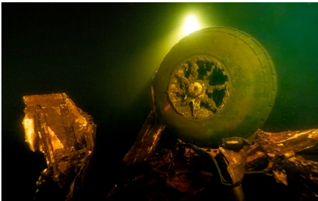
Figure 5: Nose wheel of landing gear in the extended position. Metal pieces on the left are the two nose wheel doors that close when the wheel is retracted into the fuselage after take-off. Frame from video: Jill Heinerth
