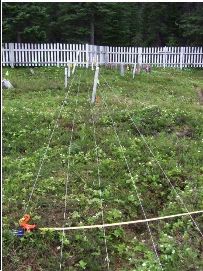
Figure 5: A grid prepared for GPR survey with measuring tape & transect lines spaced 0.25 m.
