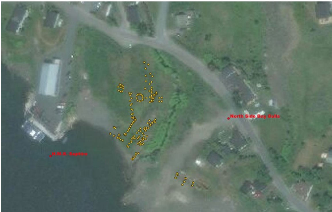
Figure 7: Closer look at Site 3, yellow dots are RTK points recorded as an indication of structures.
