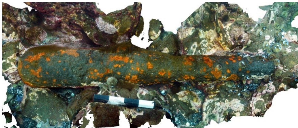
Figure 7: 3D photogrammetry image of cannon 3 at Garrison Point, Little Mortier Guns site (CgAs-1). Each unit of the scale bar is 10-cm. 3D model: Neil Burgess SPSNL. View the interactive 3D model at https://skfb.ly/oE9WN
