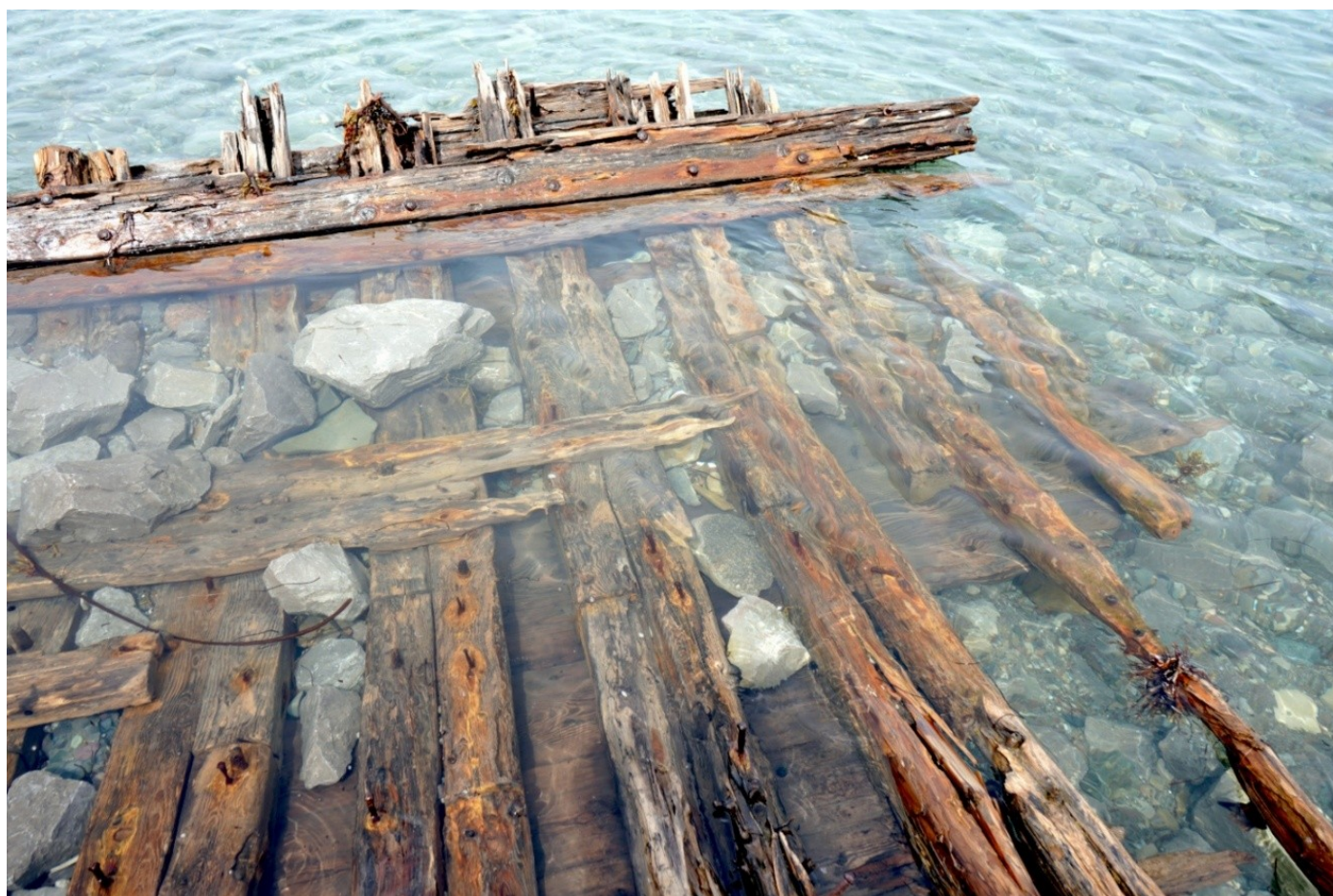
Figure 3: Shoal Point shipwreck showing the external hull planking underneath, paired framing timbers in the middle, and a few internal ceiling planks on top (most are missing). Note the spaces between the paired frames. The bottom of the photo is close to the keel and the turn of the bilge is at the top. photo: Neil Burgess SPSNL
