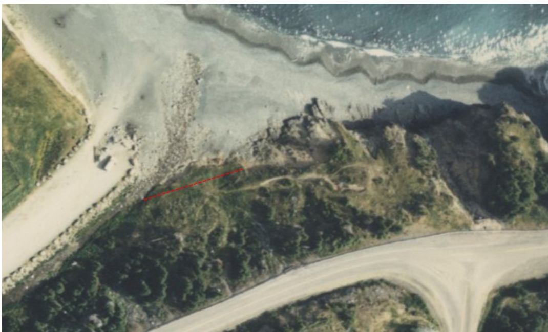
25.29 Figure 2: Aerial image of Middle Cove Beach from 1987. The red line shows the approximate quantity of erosion in the subsequent c. 38 years (when compared to modern aerial photos).
