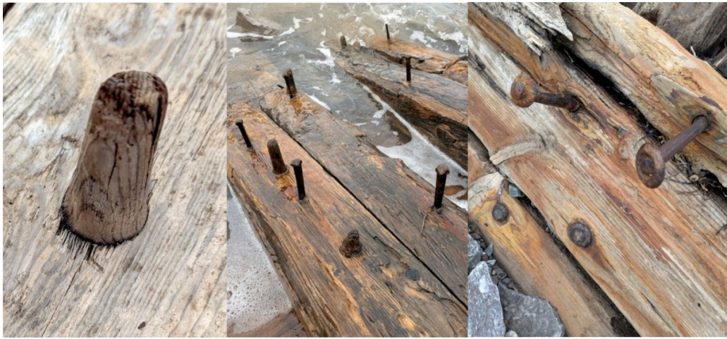
Figure 4: Fasteners in the Shoal Point shipwreck. A wooden treenail on the left, treenails and square-sectioned iron spikes in the centre, and wrought-iron through bolts with hammered heads securing clinch rings on the right. photos: Patrick Ballett
