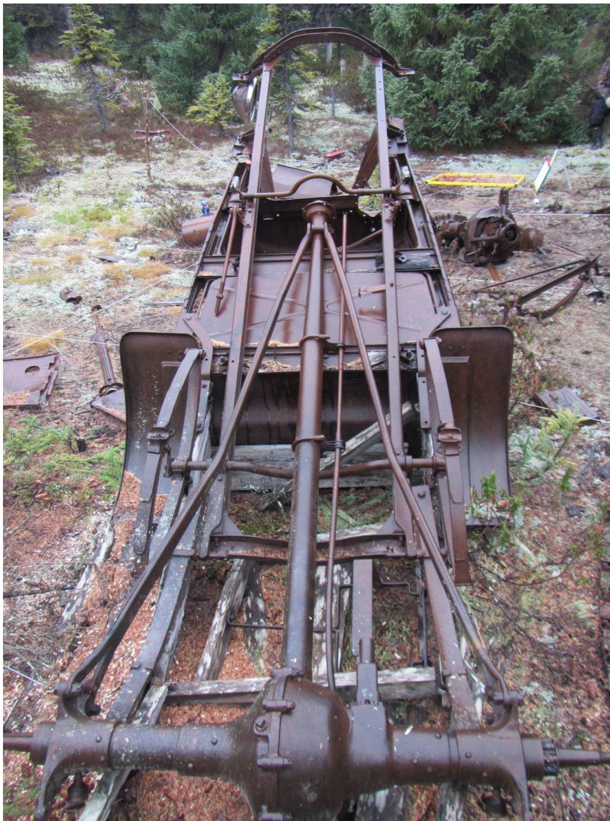
Figure 7. Underside of the snowmobile on October 19 th , 2013. Note the condition of the metal, and of the chassis in particular.
