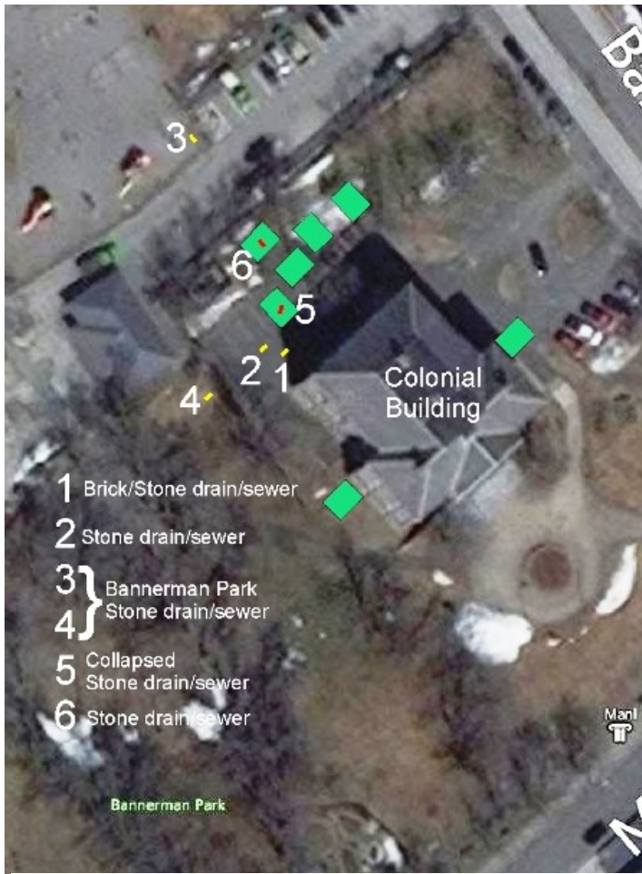
Figure 19. The yellow rectangles are brick/stone drains found during construction. The green rectangles are PAO tractor excavated test trenches, the red rectangles are brick/stone drains found in the PAO test trenches.
