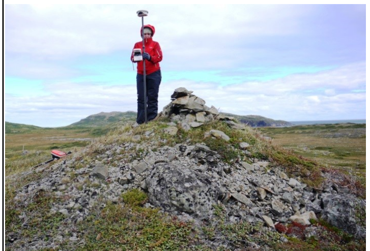
Figure 2 Photograph of rover antenna (Leica GS09 GNSS) with hand held unit (CS09 Controller). Photo: CARRA Project.
