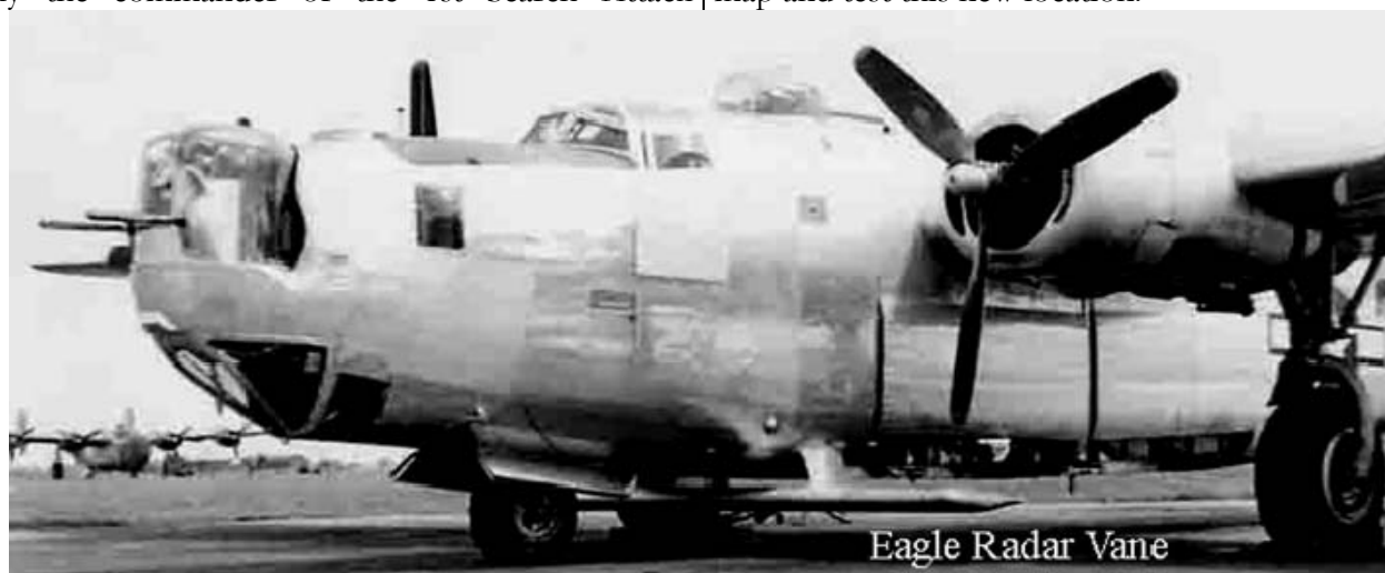
Figure 1: Eagle bomber with radar device housed in an airfoil-shaped cover, suspended beneath the nose of the aircraft. (Deal)
