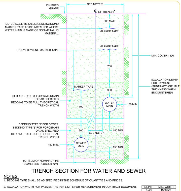
3. UNDER NO CIRCUMSTANCES, SHALL ANY FORCEMAIN BE INSTALLED AT ZERO SLOPE.
