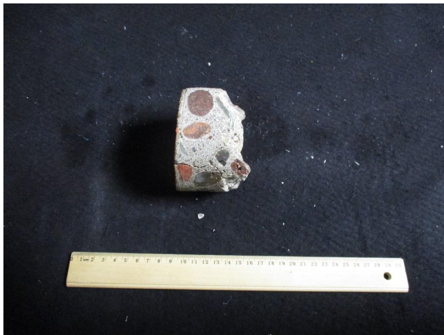
Core 32 Sampled from Swing Pier – Top face
