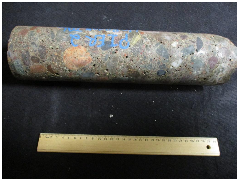
Core 21 Sampled from Pier 2 - Above high-water line
