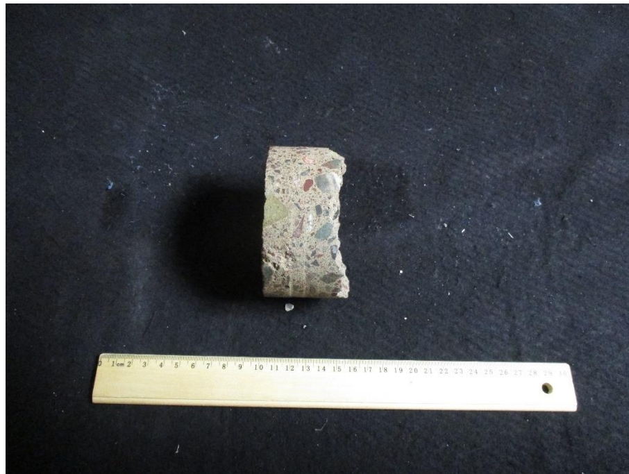
Core D8 Sampled from Bridge Deck
