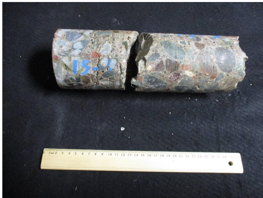
Core 15 Sampled from North Abutment – Back Wall
