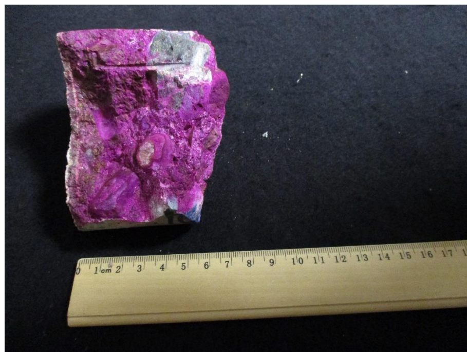
Core 32 - Carbonation Depth Sampled from Swing Pier - Top face
