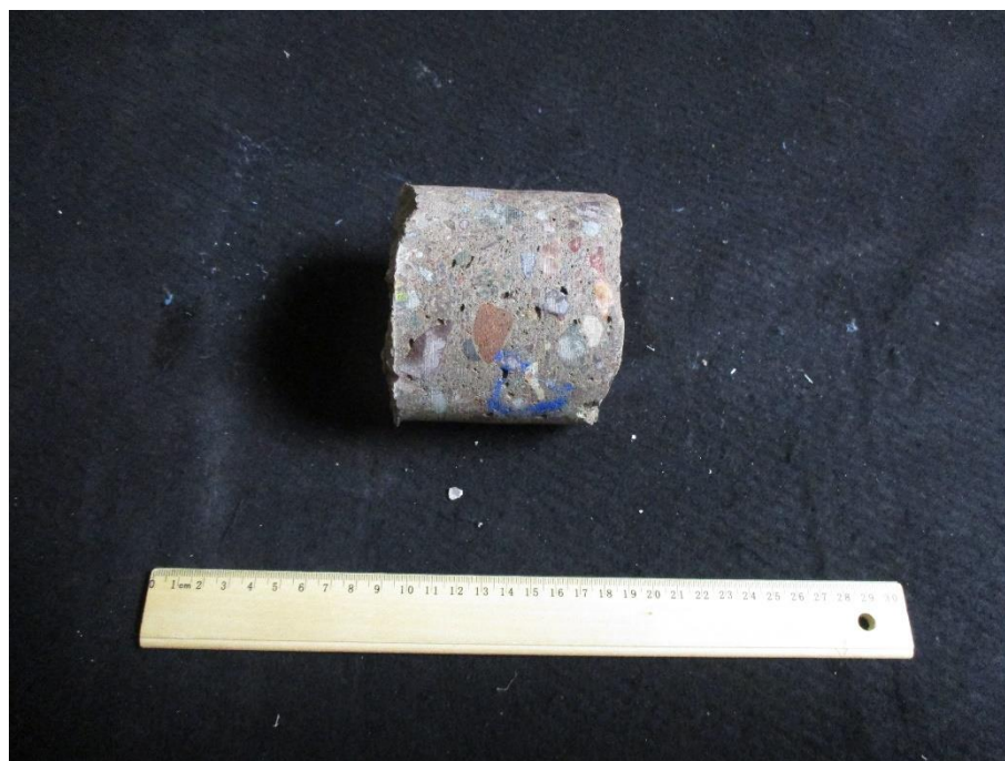
Core D9 Sampled from Bridge Deck
