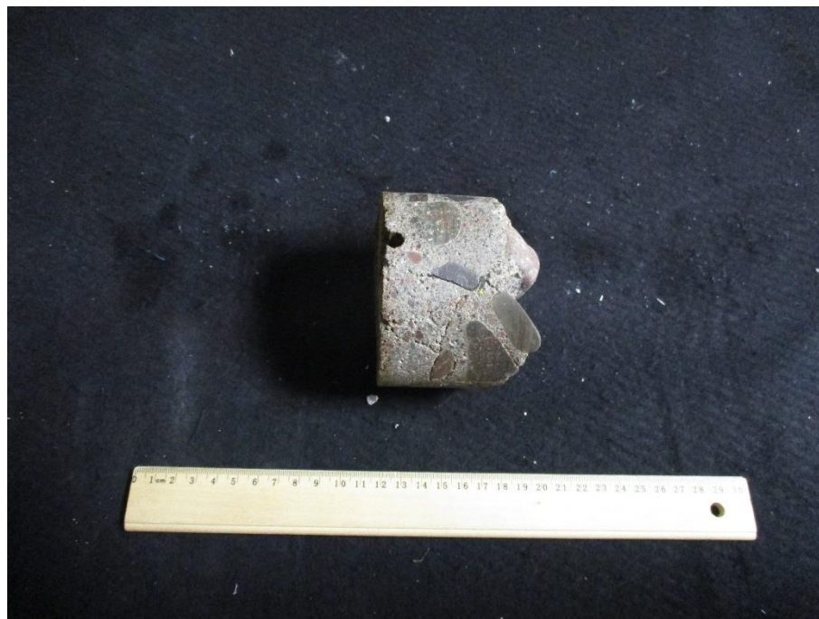
Core 31 Sampled from Swing Pier - Top face
