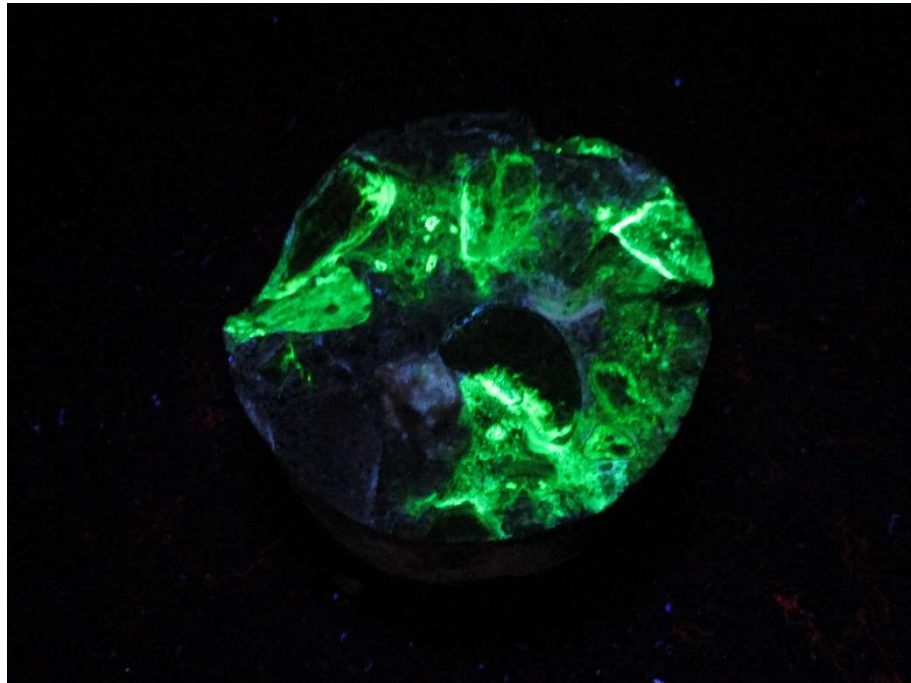
Core 9 Under UV Light following Exposure to Uranyl Acetate Solution
