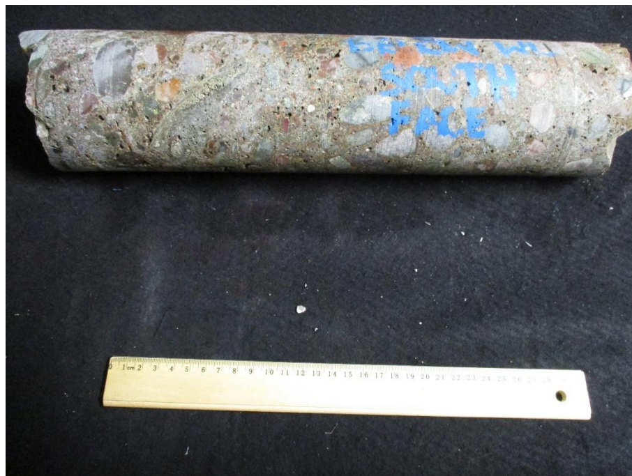
Core 26 Sampled from Pier 1 – Below high-water line in tidal zone
