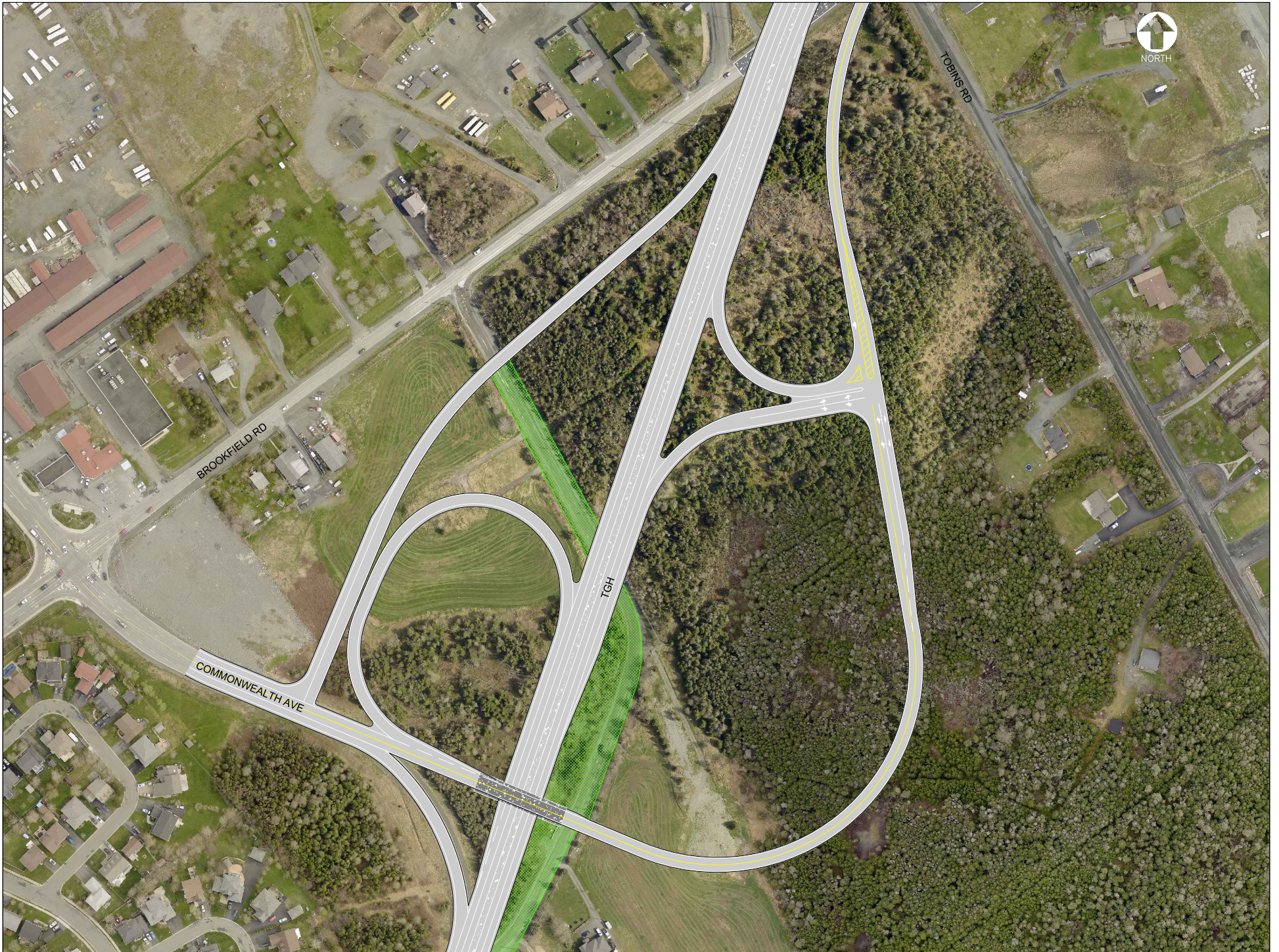
Figure 3: Grade Separated Interchange Connection - Concept Drawing
