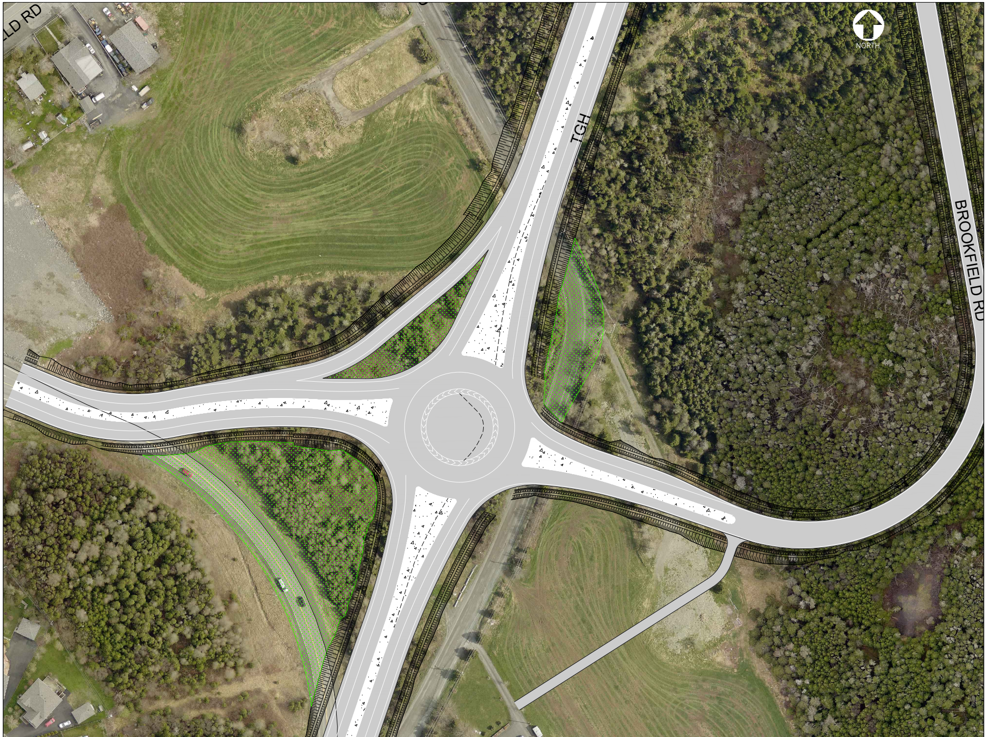
Figure 2: At-Grade Roundabout Connection - Concept Drawing
