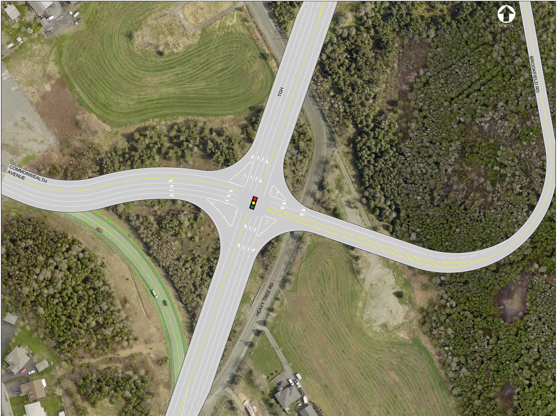
Figure 1: At-Grade Signalized Intersection Connection - Concept Drawing
