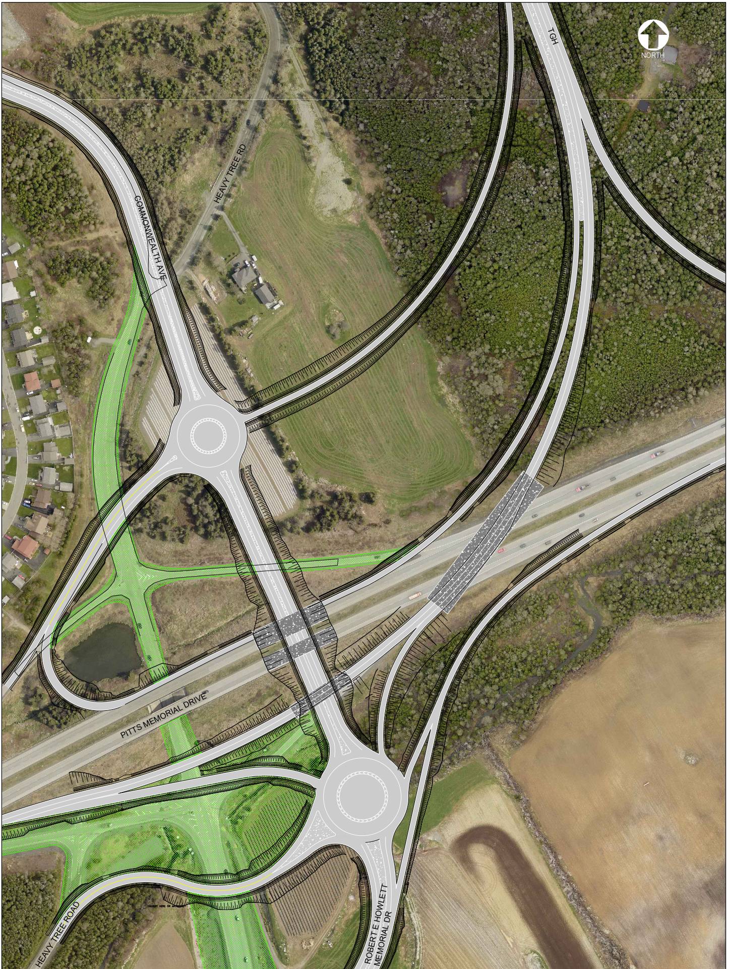
Figure 13: Option 5 Route 2/Route 3 Interchange Flyover – Detailed Concept
