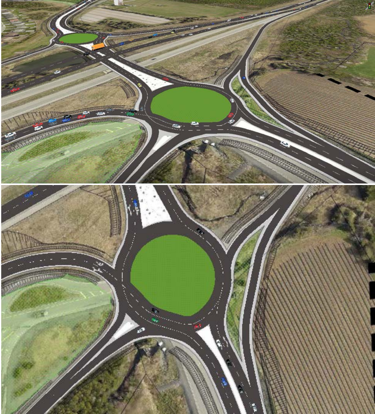
Figure 16: Microsimulation Model Circulatory Lanes
