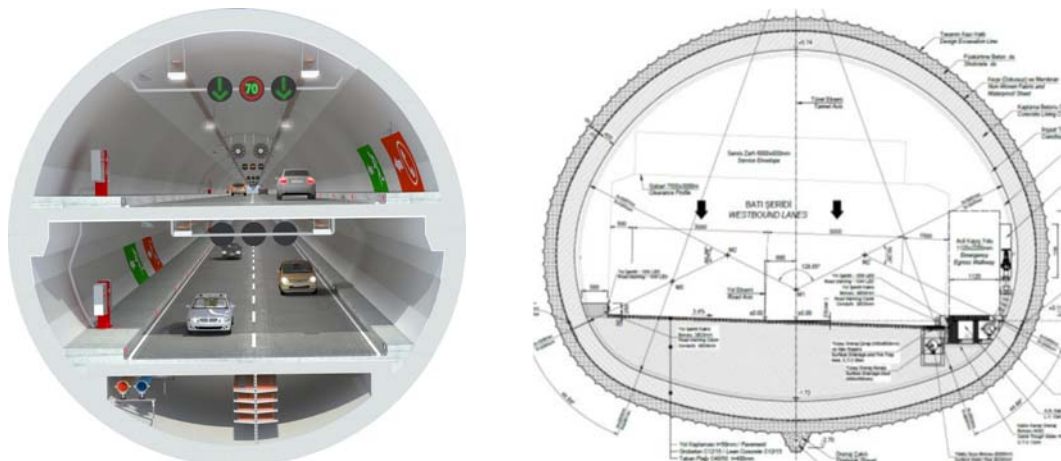
Figure 4-3: Eurasia Tunnel Cross Sections: TBM (left), Drill & Blast (right) ( https://www.newcivilengineer.com/world-view/under-pressure-eurasia-tunnel/10001844.article ); (Istanbul Strait Road Tube Crossing: Challenges, Risk and Mitigation Strategies, N. Munfah et al.)
